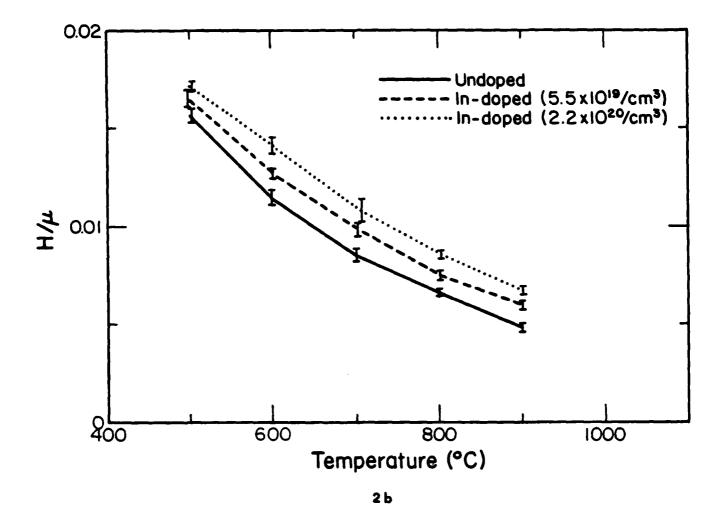
2. Normalised hardness versus temperature plot for GaAs, Ga<sub>.9975</sub>In<sub>.0025</sub>As and Ga<sub>.99</sub>In<sub>.01</sub>As.
