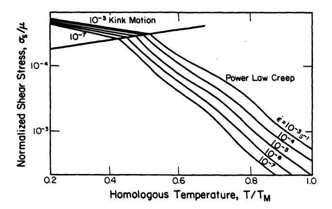
4. A section of deformation mechanism map of Si which belongs to the same iso-mechanical group as GaAs.<sup>19</sup>
