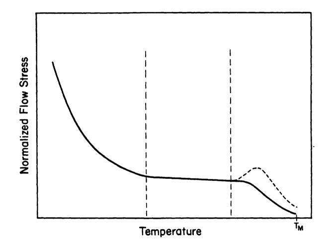
1. Schematic normalised flow stress versus temperature curve for GaAs at
