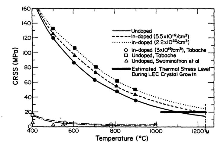
3. Critical resolved shear stress estimated from hardness data compared with the compression test data of Swaminathan and Copely<sup>15</sup> on undoped GaAs and of Tabache<sup>16</sup> on undoped and In-doped LEC GaAs.
