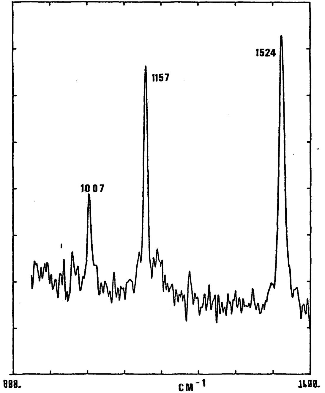
Figure 1 The resonance Raman spectrum of intact turtle cone oil droplets with 520.8 nm excitation
