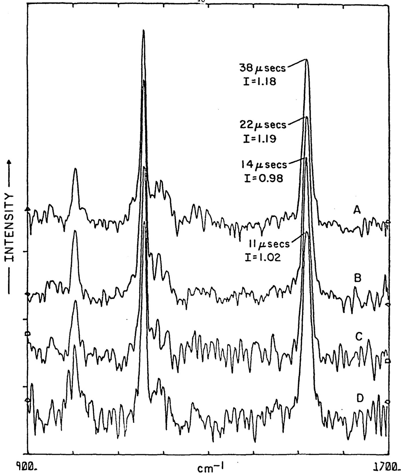
Figure 4 Kinetic resonance Raman spectroscopy of carotenoids in turtle retina with various time delays after a stimulating light pulse. Spectra were taken with 514.5 nm excitation and I = intensity ratio of the 1157 cm<sup>-1</sup> band to the 1520 cm<sup>-1</sup> band.
