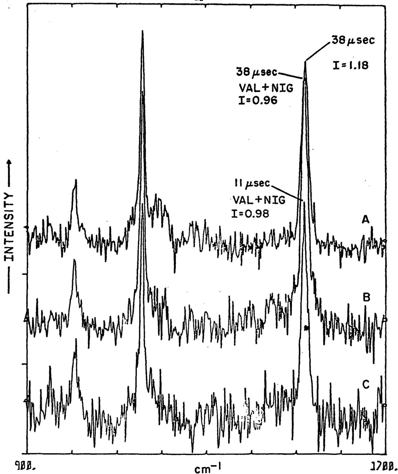
Figure 5 A comparison of the kinetic resonance Raman spectra of carotenoids in turtle retina obtained with a 38  $\mu\text{s}$  delay after light excitation (A) without and (B) with valinomycin and nigericin and at 11  $\mu\text{s}$  with valinomycin and nigericin (C). Spectra obtained with the same laser frequency and I has the same definition as in Figure 4.
