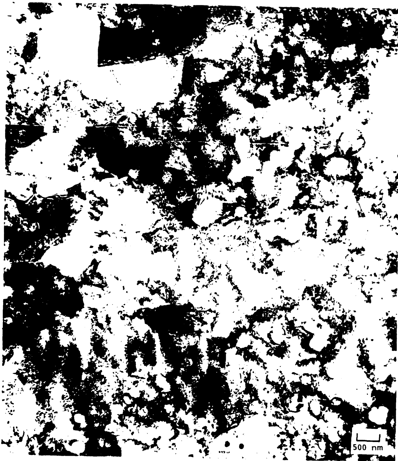
Fig. D11. Al-3Li-10Be consolidated alloy in the T6 condition after testing.
