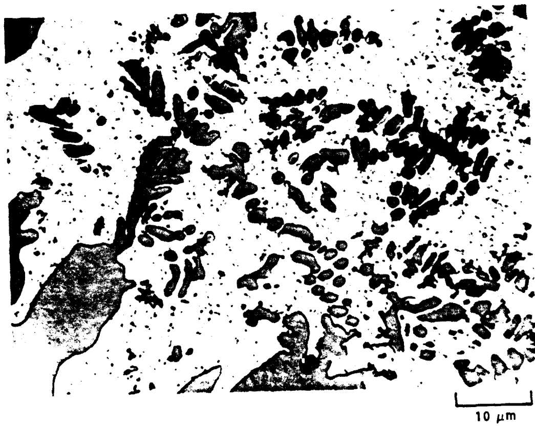
Fig. B1 (a) Splat quenched sample. (b) Microstructural variation within a splat quenched Al-3Li-10Be alloy.
