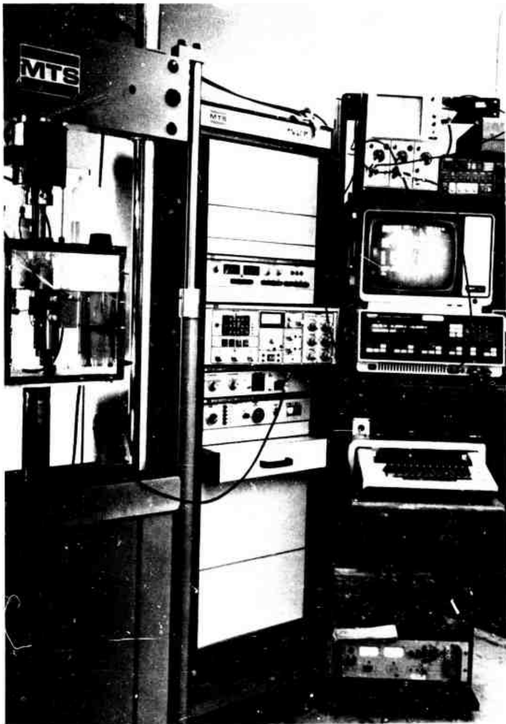
FIGURE 13 FACILITY FOR MEASURING IMPEDANCE SPECTRA OF STRESS CORROSION CRACKING OR CORROSION FATIGUE TEST SPECIMENS
