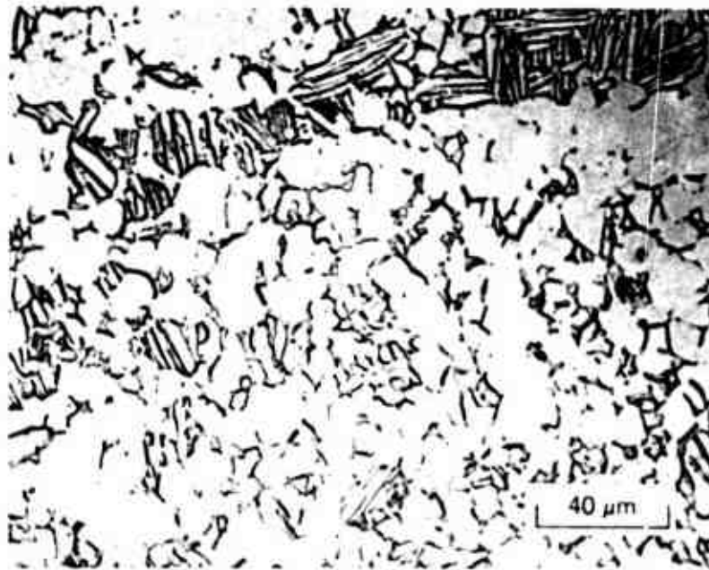
(b) Ti-6Al-4V (Looking onto plane of crack path)
