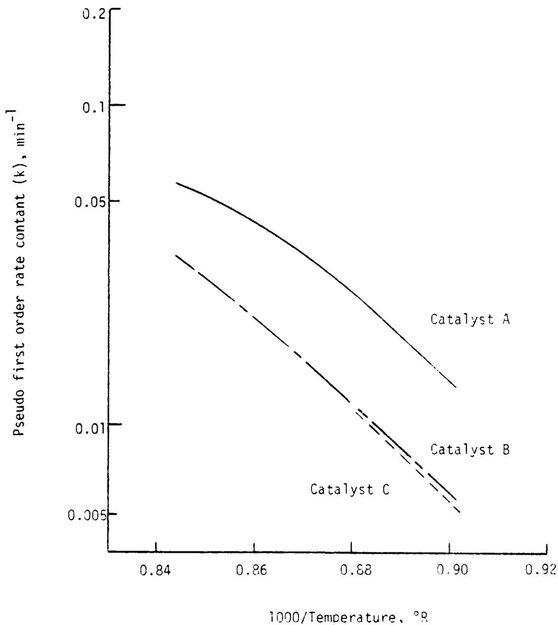
FIGURE 3 COMPARISON OF CATALYST ACTIVITIES FOR HYDRODENITROGENATION REACTION
