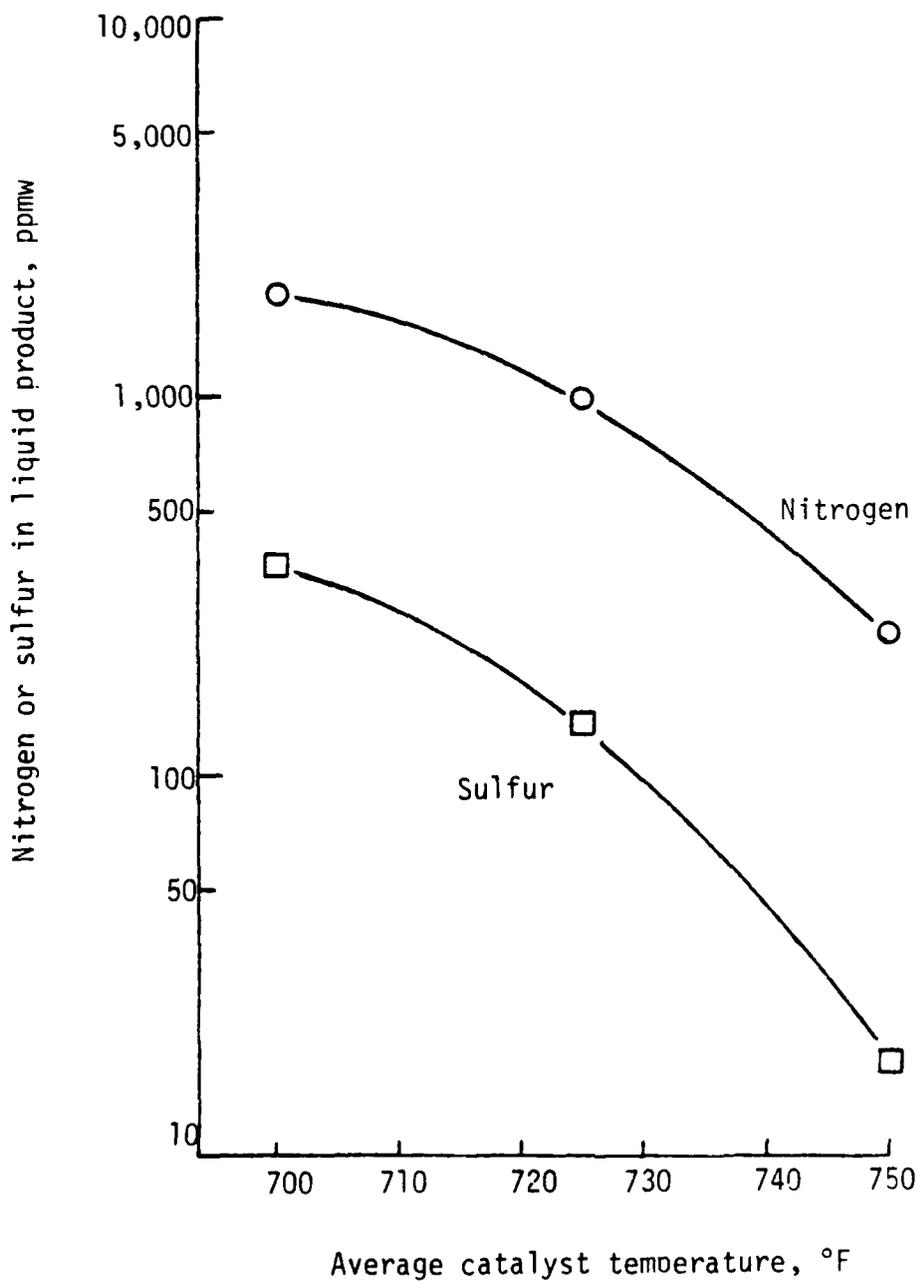
FIGURE 15 HYDROTREATING SAN ARDO DISTILLATE;
