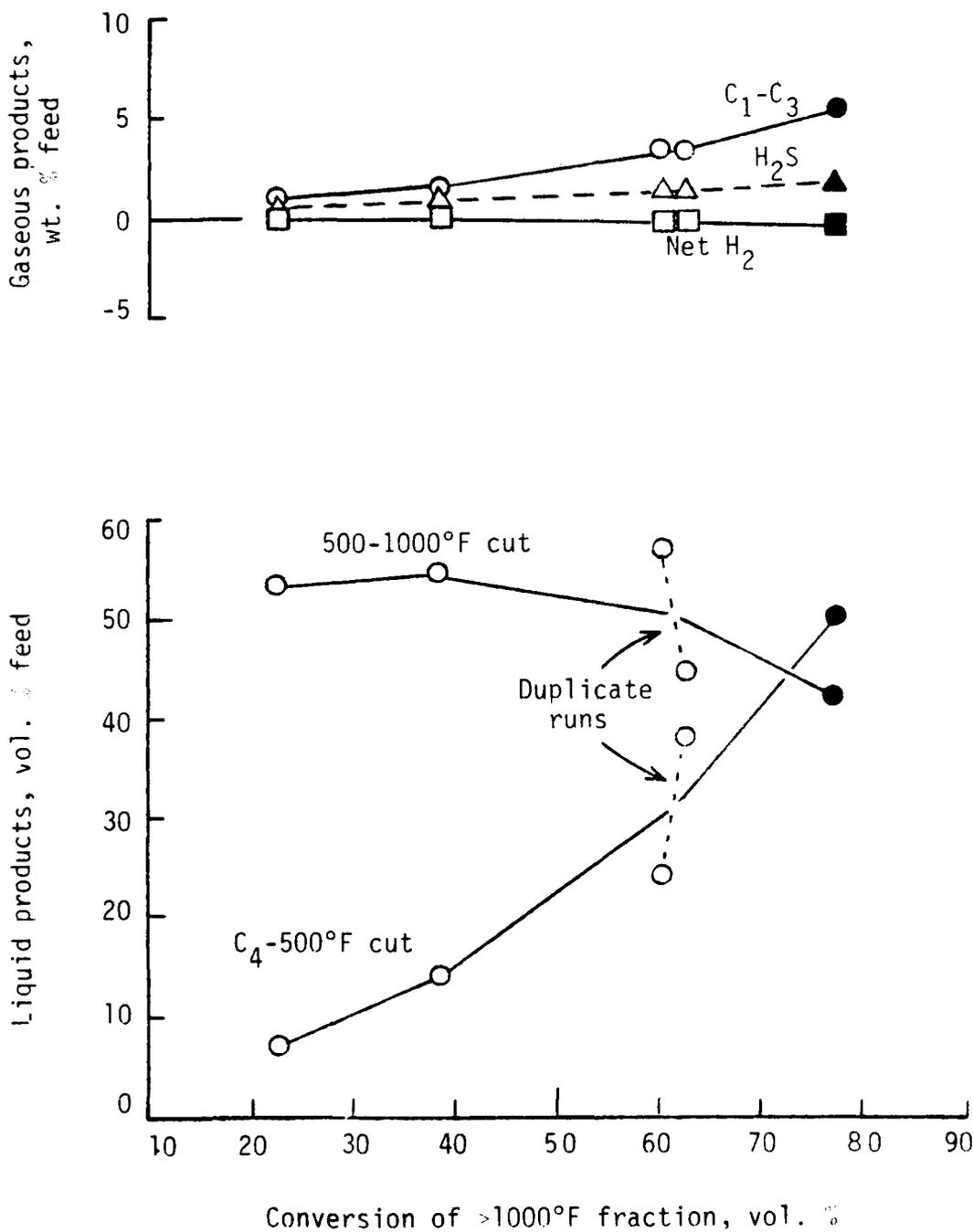
FIGURE 9 BATCH HYDROVISBREAKING OF SAN ARDO >650°F FRACTION
