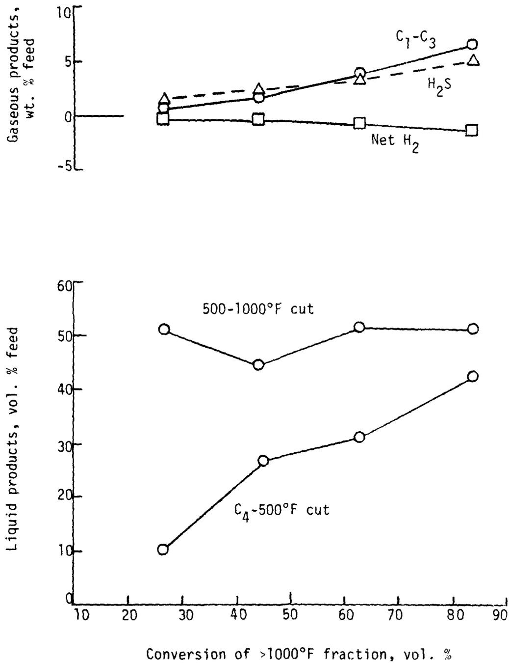
FIGURE 8 BATCH HYDROVISBREAKING OF HONDO MONTEREY >650°F FRACTION
