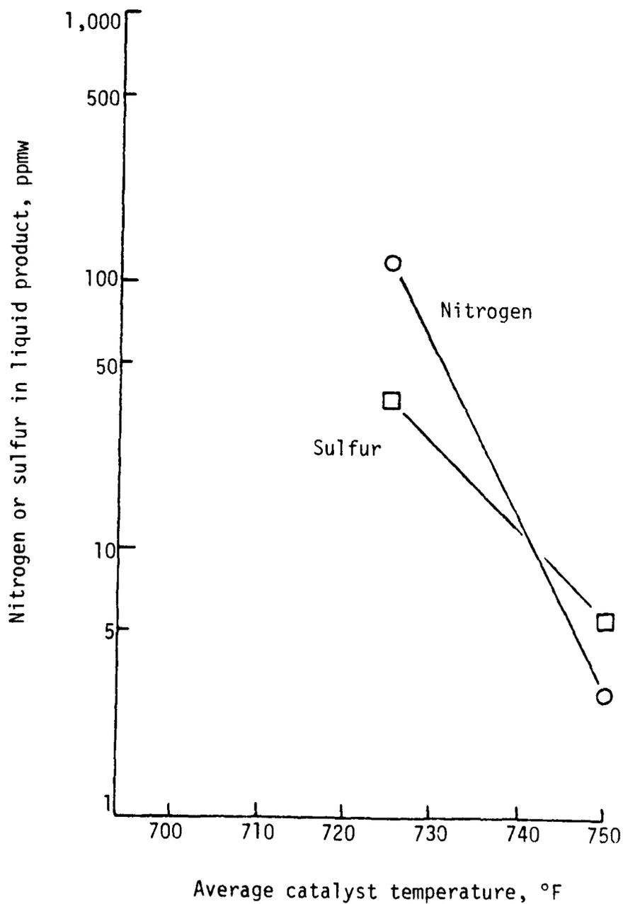
FIGURE 18 HYDROTREATING KENSYNTAR DISTILLATE
