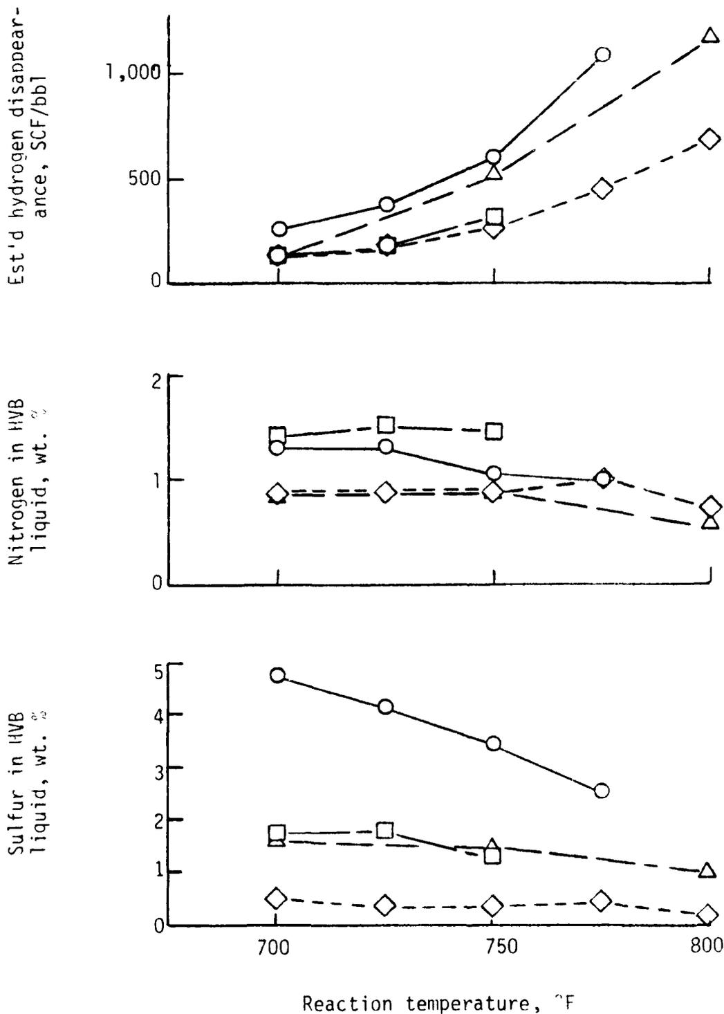
FIGURE 6 TEMPERATURE EFFECTS IN BATCH HYDROVISBREAKING
