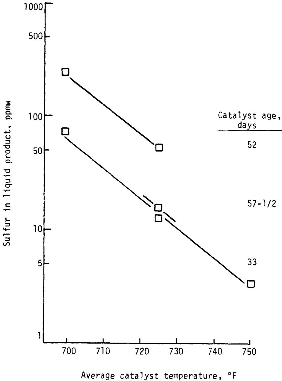
FIGURE 14 HYDROTREATING HONDO MONTEREY DISTILLATE;
