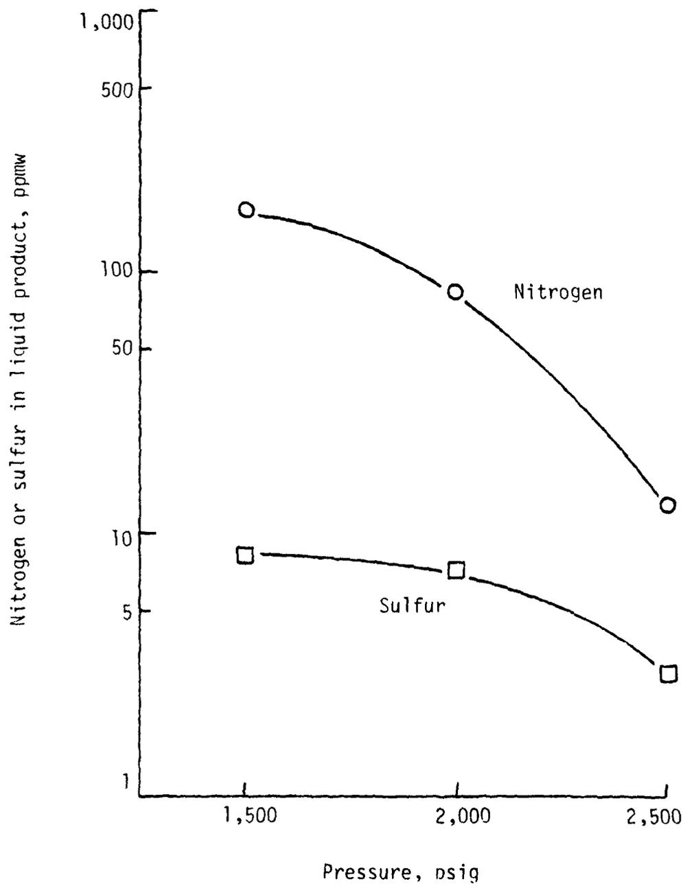
FIGURE 16 HYDROTREATING SAN ARDO DISTILLATE;
