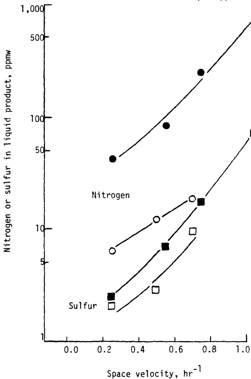
FIGURE 17 HYDROTREATING SAN ARDO DISTILLATE;
