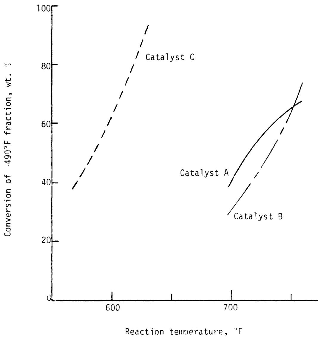
FIGURE 4 COMPARISON OF HYDROCRACKING CATALYST ACTIVITIES
