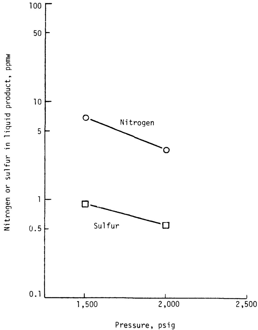
FIGURE 22 HYDROTREATING SUNNYSIDE DISTILLATE;
