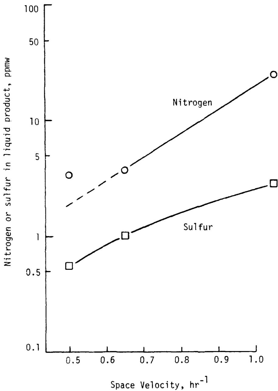
FIGURE 21 HYDROTREATING SUNNYSIDE DISTILLATE;
