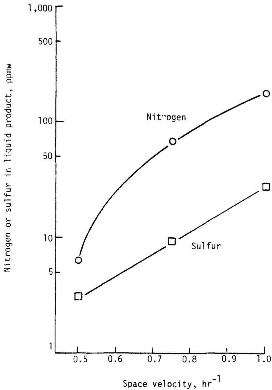
FIGURE 19 HYDROTREATING KENSYNTAR DISTILLATE;
