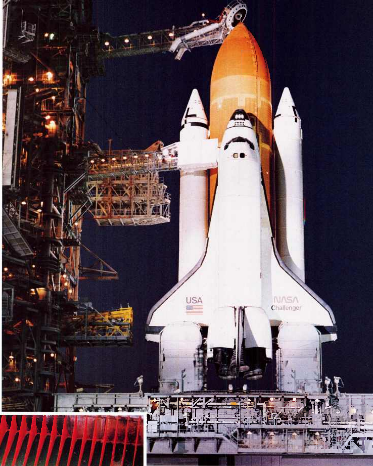
Above, Shuttle 51-L on Kennedy Space Center Pad 39B in the early morning of launch day. Temperatures were well below freezing, as indicated by the lower left photo, which shows thick ice in a water trough despite use of an anti-freeze solution.
