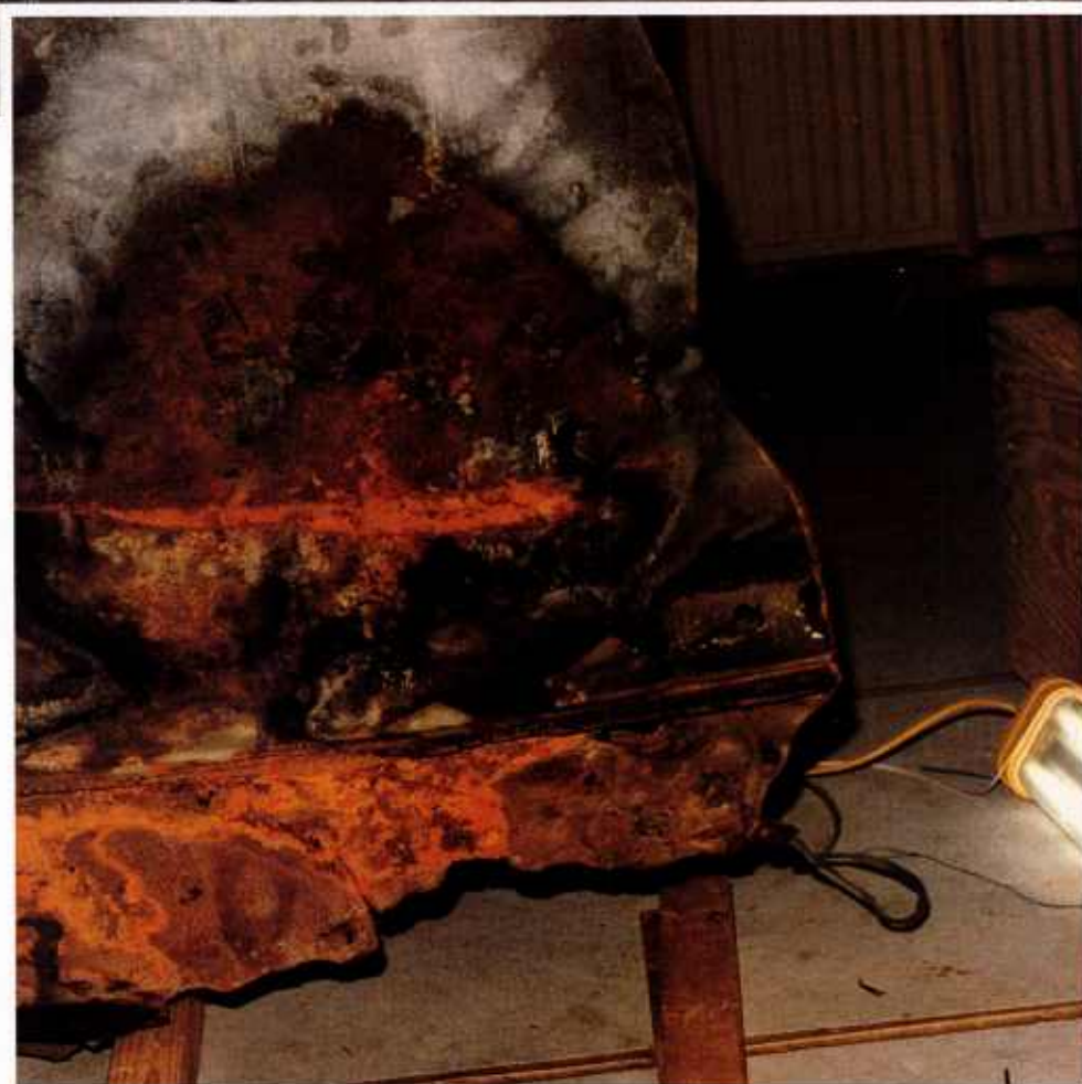
L Examined at Kennedy Space Center after their recovery from the ocean, these fragments show the extent of burn through the right hand booster's aft field joint. On the left page are sections of the aft center motor segment above the joint. On the right page are sections (inverted) of the aft motor segment showing burn-hole below the joint (bracket). Except for the interior views on lower left, the camera is viewing the parts from outside the casing.
