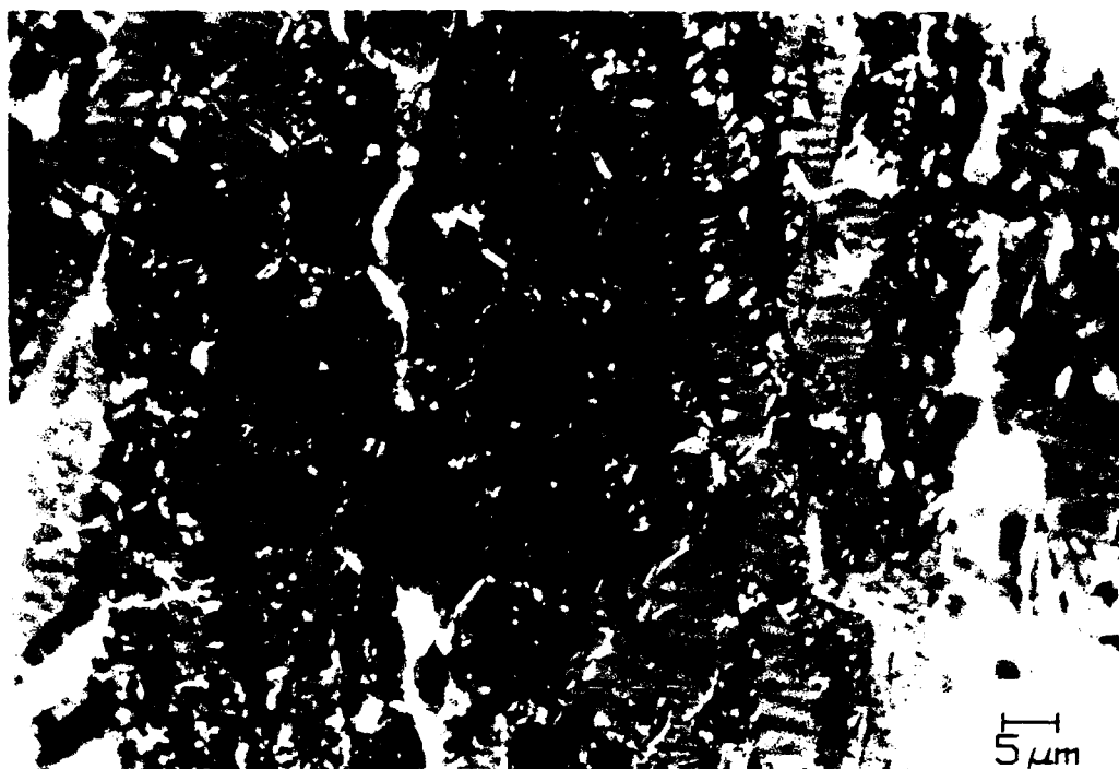
Figure 3-5. Large multiphase particle produced in run RD-4. Polarized light.
