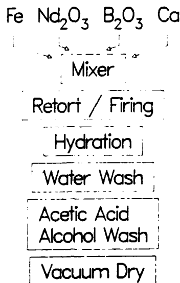
Figure 3-1. Steps in R-D process used to produce \text{Fe}_{14}\text{Nd}_2\text{B} .
