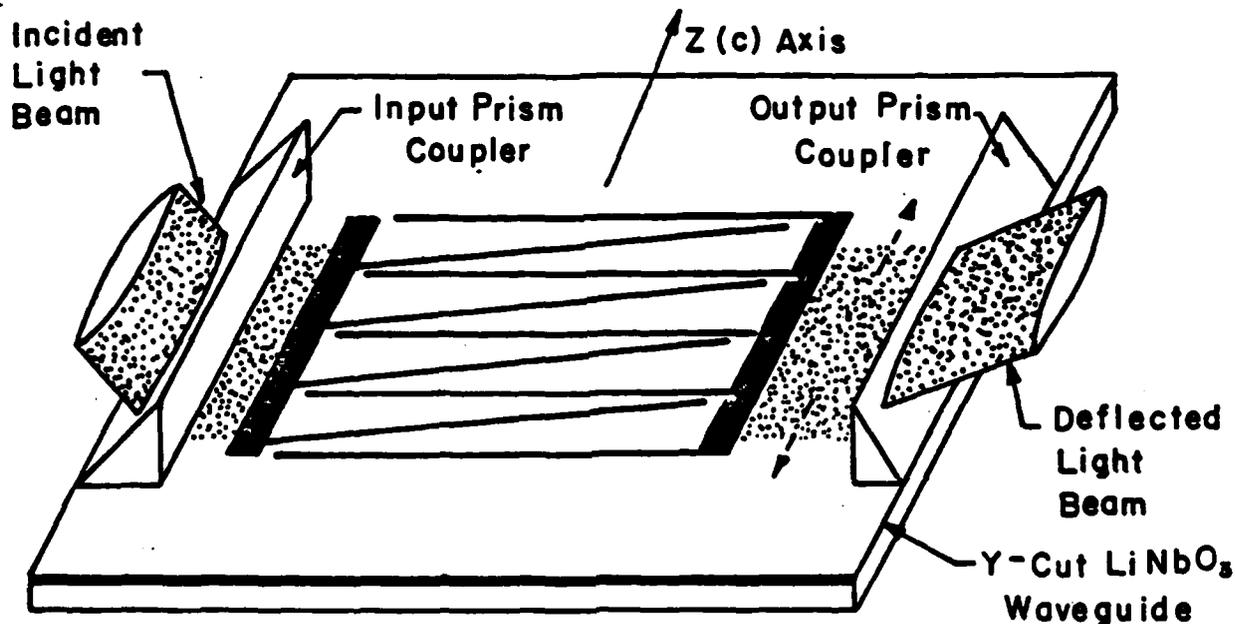
$L=1.3\text{cm}$ ,  $H=150\mu\text{m}$ ,  $h=5\mu\text{m}$ , Total Aperture =  $600\mu\text{m}$
