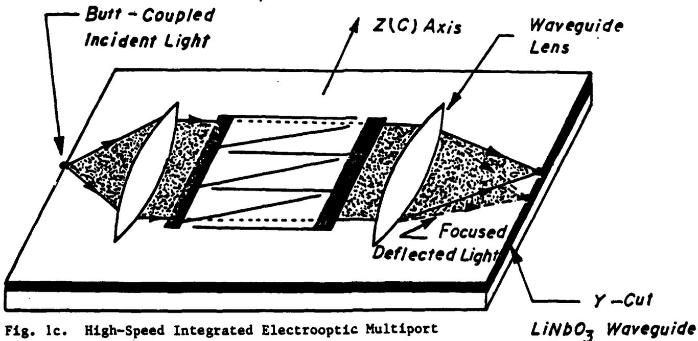
Fig. 1c. High-Speed Integrated Electrooptic Multiport Deflector/Switch Module
