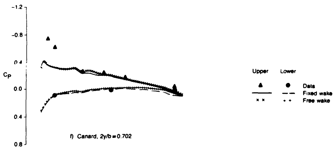
Figure 8. Data-analysis pressure comparison, CDAF, Mach 0.9, \alpha 7.0 (sheet 2 of 2).
