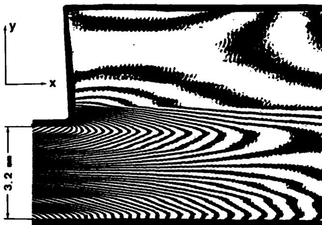
x-displacement field near the corner of an adhesive joint between two graphite-epoxy composite plates subjected to bending. Sensitivity corresponds to moire with 2400  $\lambda$ /mm (60,960  $\lambda$ /in.).
