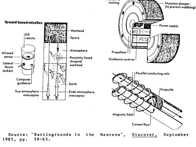
FIGURE 9. Proposed Beam and Kinetic Energy Weapons
