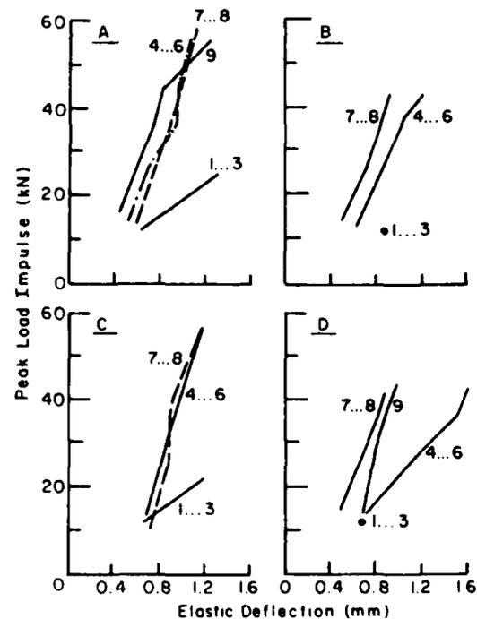
Figure 12. Elastic deflections of reinforced beams prior to cracking of the concrete. See Table 1 to identify reinforcement types for groups A, B, C and D.
