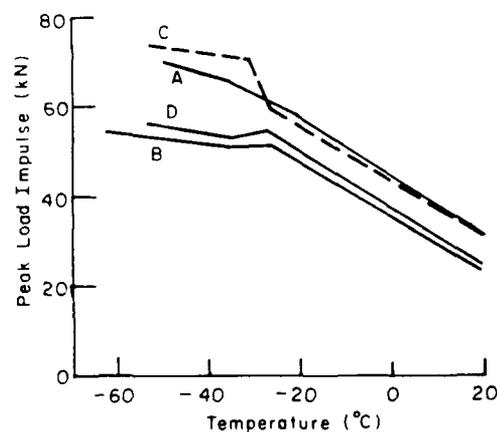
Figure 7. Loads at which reinforced beams first cracked.
