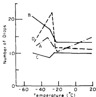
Figure 5. Drops needed to break tension reinforcement (see Table 1 for beam group designations.)
