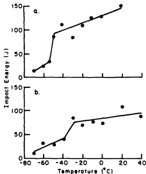
Figure 13. Relationship between failure energy and temperature for the steels in the Charpy-V test. a-cold worked smooth bar, b-hot rolled deformed bar.
