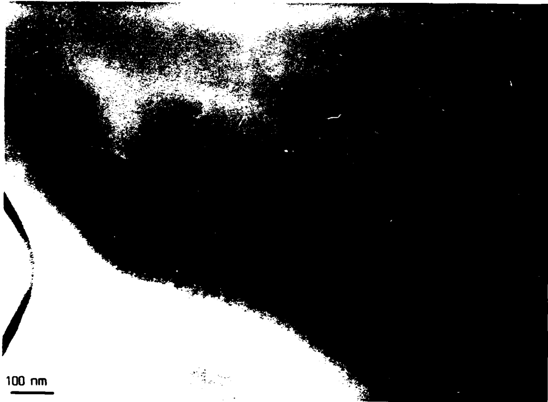
Fig.15: Electron micrograph showing a grain boundary layer phase separating two hard magnetic grains. An increased Si-content is found by at the grain boundary region.
