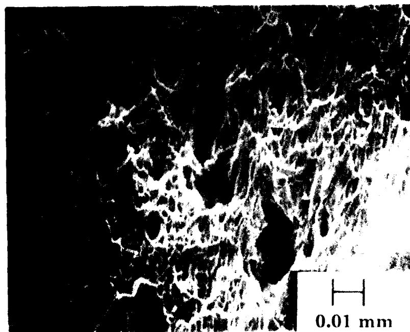
Figure 9: SEM Photographs of the Fracture Surface, 1215 Steel 2
