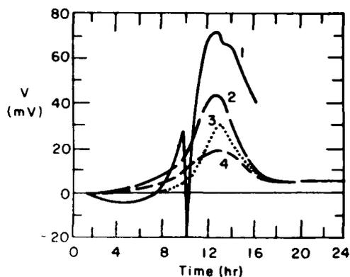
Figure 2. Change of electrical potential difference during the process of freezing sand with different spacings between the electrodes (1: 20 mm; 2: 10 mm; 3: 5 mm; 4: 2.5 mm).
