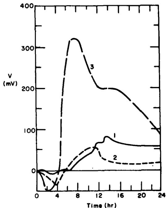
Figure 1. Change of electrical potential difference during freezing of samples of sandy soils (1 - sand with 20% moisture content; 2, 3 - powdered sand with moisture content 19.8 and 22.7%).
