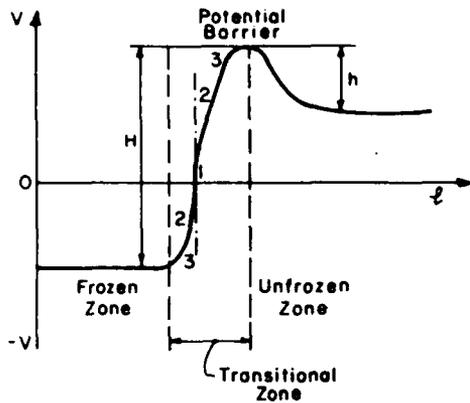
Figure 4. Schematic diagram of the electric charge distribution along the profile of a sample of freezing sand. (1, 2, 3 - regions of potential jump, linear, and nonlinear change in potential.  $H$  and  $h$  are the heights of the potential barrier in the frozen zone and the non-frozen zone respectively; the dash-dot line marks the freezing boundary.)
