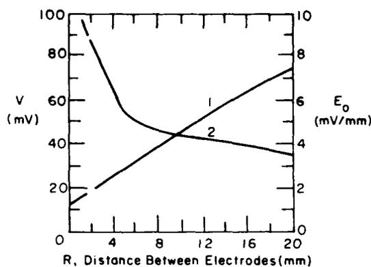
Figure 3. Variation of the difference (curve 1) and the gradient of electrical potentials (curve 2) with change of spacing between the electrodes.
