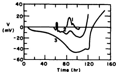
Figure 7. Change in electrical potential difference during the freezing of samples of kaolin at different rates of freezing (1, 2, 3 - freezing rates of 5, 4 and 0.6 mm/hr, respectively).
