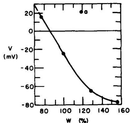
Figure 6. Dependence of maximum electrical potential difference on the moisture content of freezing samples of bentonite (a - result of tests with bentonite of particle size  $< 0.001$  mm).
