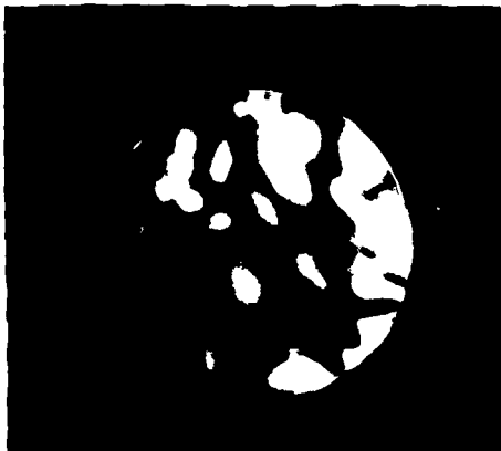
Figure 1. Intensity-scintillation pattern of a 0.63- \mu\text{m} spherical wave 1012 m from its source. The pattern is 50 mm in diameter, the exposure is 1/2000 s with winds less than 1 m/s, and C_n^2 = 3 \times 10^{-13} .
