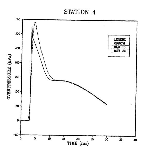
Figure 41. Comparison of Overpressure From the Original and the Revised BOUND9 Coding at Station  $^4\cdot$
