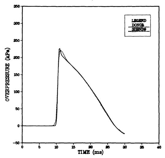
Figure 19. Comparison of Overpressure From a 2-D Donor Run and a 3-D Imposed-Boundary Run for a 20 cm Mesh at Station 6.
