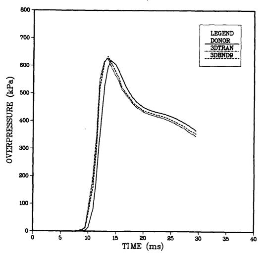
Figure 3. Comparison of Overpressure From a 2-D Donor Run, a Comparative 3-D Run, and a 3-D Imposed-Boundary Run for an 80 cm Mesh at Station 2.
