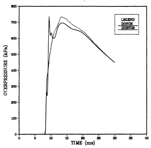
Figure 20. Comparison of Overpressure From a 2-D Donor Run and a 3-D Imposed-Boundary Run for a 10 cm Mesh at Station 1.
