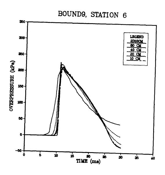
Figure 37. Overpressure From Imposed-Boundary Runs at Station 6.
