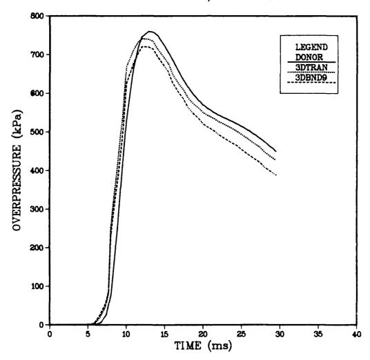
Figure 2. Comparison of Overpressure From a 2-D Donor Run, a Comparative 3-D Run, and a 3-D Imposed-Boundary Run for an 80 cm Mesh at Station 1.
