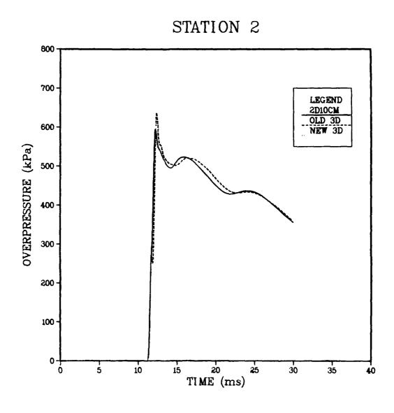
Figure 39. Comparison of Overpressure From the Original and the Revised BOUND9 Coding at Station 2.
