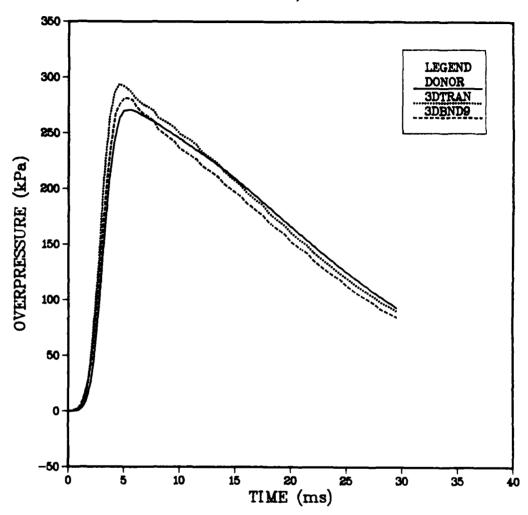
Figure 5. Comparison of Overpressure From a 2-D Donor Run, a Comparative 3-D Run, and a 3-D Imposed-Boundary Run for an 80 cm Mesh at Station 4.
