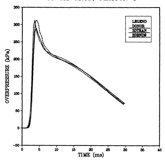
Figure 11. Comparison of Overpressure From a 2-D Donor Run, a Comparative 3-D Run, and a 3-D Imposed-Boundary Run for a 40 cm Mesh at Station 4.
