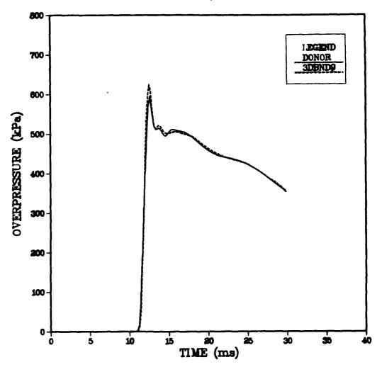
Figure 15. Comparison of Overpressure From a 2-D Donor Run and a 3-D Imposed-Boundary Run for a 20 cm Mesh at Station 2.
