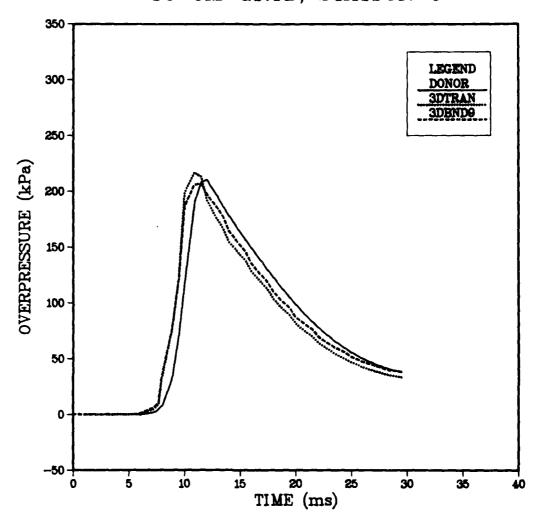
Figure 7. Comparison of Overpressure From a 2-D Donor Run, a Comparative 3-D Run, and a 3-D Imposed-Boundary Run for an 80 cm Mesh at Station 6.
