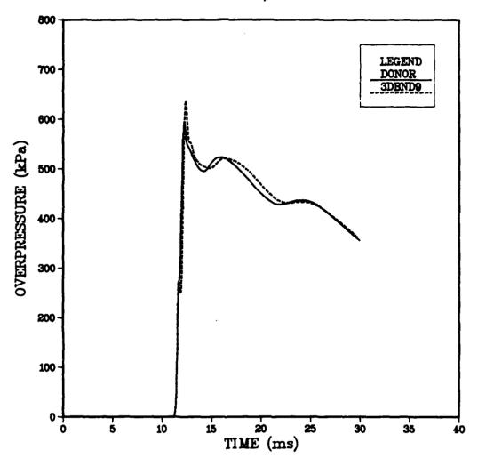
Figure 21. Comparison of Overpressure From a 2-D Donor Run and a 3-D Imposed-Boundary Run for a 10 cm Mesh at Station 2.
