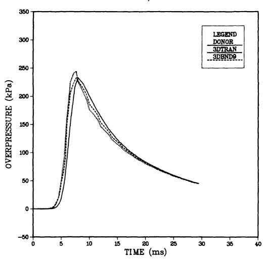
Figure 6. Comparison of Overpressure From a 2-D Donor Run, a Comparative 3-D Run, and a 3-D Imposed-Boundary Run for an 80 cm Mesh at Station 5.
