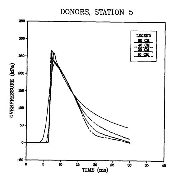
Figure 30. Overpressure From 2-D Donor Runs at Station 5.
