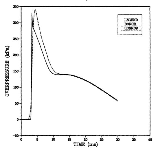
Figure 23. Comparison of Overpressure From a 2-D Donor Run and a 3-D Imposed-Boundary Run for a 10 cm Mesh at Station 4.
