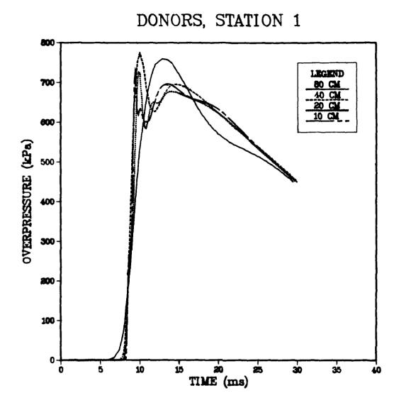
Figure 26. Overpressure From 2-D Donor Runs at Station 1.
