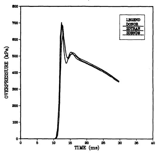
Figure 9. Comparison of Overpressure From a 2-D Donor Run, a Comparative 3-D Run, and a 3-D Imposed-Boundary Run for a 40 cm Mesh at Station 2.
