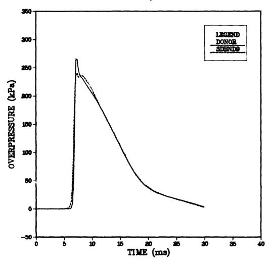
Figure 18. Comparison of Overpressure From a 2-D Donor Run and a 3-D Imposed-Boundary Run for a 20 cm Mesh at Station 5.
