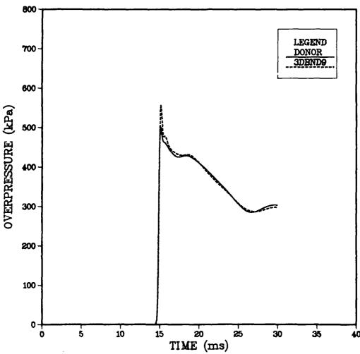
Figure 22. Comparison of Overpressure From a 2-D Donor Run and a 3-D Imposed-Boundary Run for a 10 cm Mesh at Station 3.
