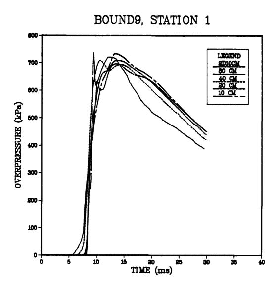
Figure 32. Overpressure From Imposed-Boundary Runs at Station 1.
