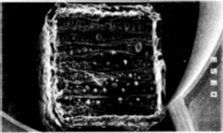
b. Cross section of the fracture surface showing deterioration of the C/C substrate, bar = 1000 μm.
