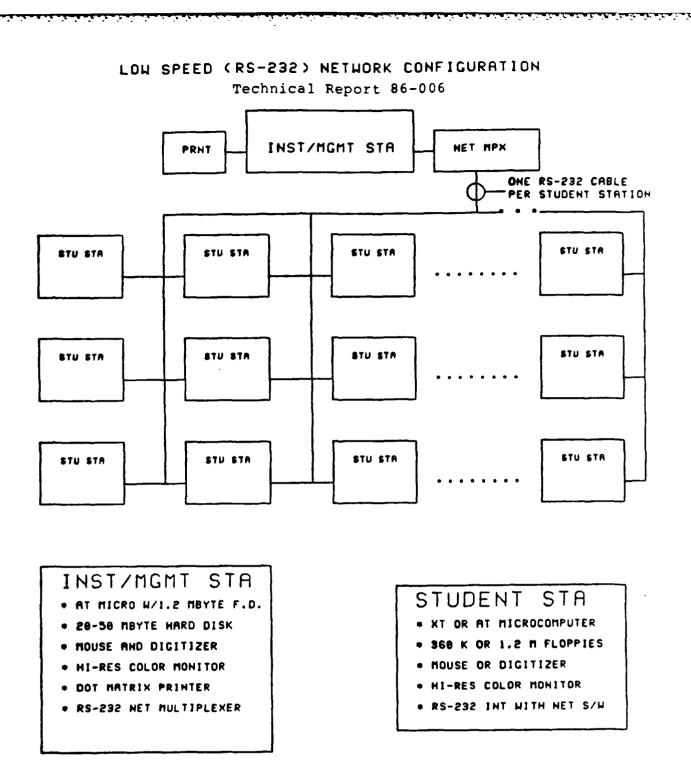
Figure 3. Instructional laboratory configuration No. 2
