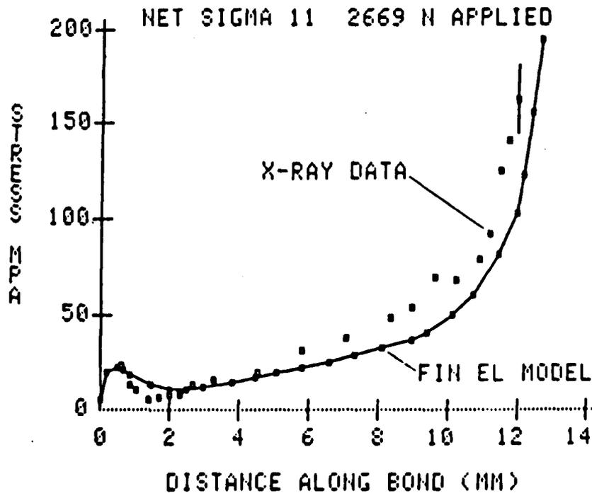
FIGURE 4 Comparison of normal stress,  $\sigma_{11}$ , measured by X-ray diffraction and calculated by the Texgap-2D finite element program (fin. el. model) along the Be/FM-73M/Al (6061-T4) single lap joint of Figure 1. Here and in Figures 5, 6 and 7 the measured and calculated stresses are in the Al adherend at a depth of 0.033 mm from the Al/adhesive interface; the edges of the Al and Be adherends are at 0 and 12.7 mm, respectively.
