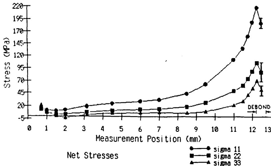
Figure 8. Net stresses  $\sigma_{11}$ ,  $\sigma_{22}$ , and  $\sigma_{33}$  due to an applied load of 2669N on specimen ARO-68 having the same dimensions as in Figure 1 except for a bond thickness of 0.069 mm and a debond 0.5 mm deep in the 1 direction at the end of the Be adherend. The Al adherend is alloy 5052 solution treated and stress relieved.
