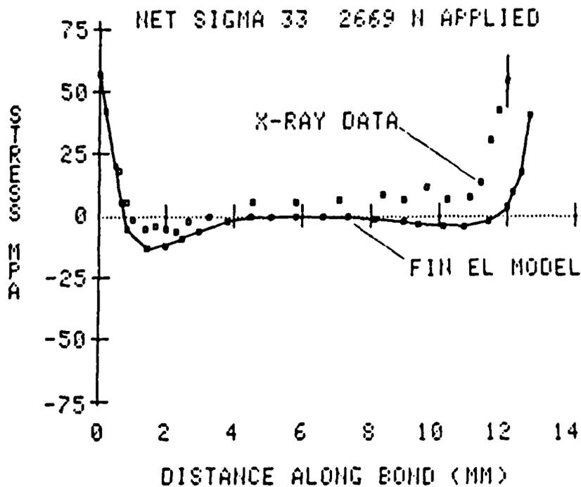
FIGURE 6 Comparison of normal peel stress  $\sigma_{33}$  measured by X-ray diffraction and calculated by the Texgap-2D program along the Bc/FM-73M/Al (6061-T6) single lap joint of Figure 1.
