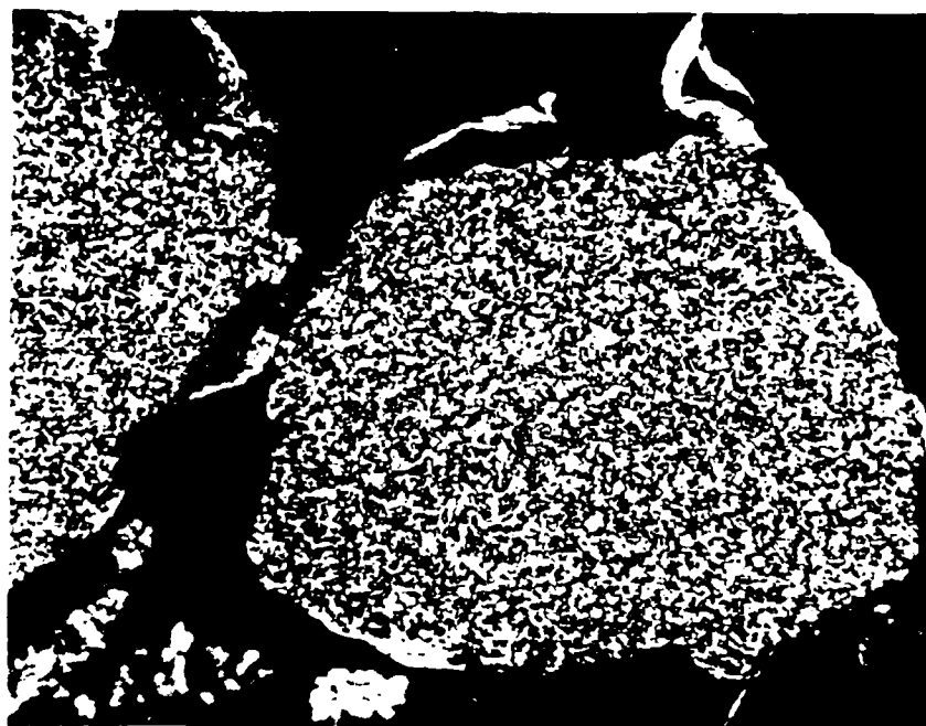
Figure 2a. Cross Sections of Aluminum - 3.0 wt.% Zr/SiC. Precomposited Powders. Magnification (500X)
