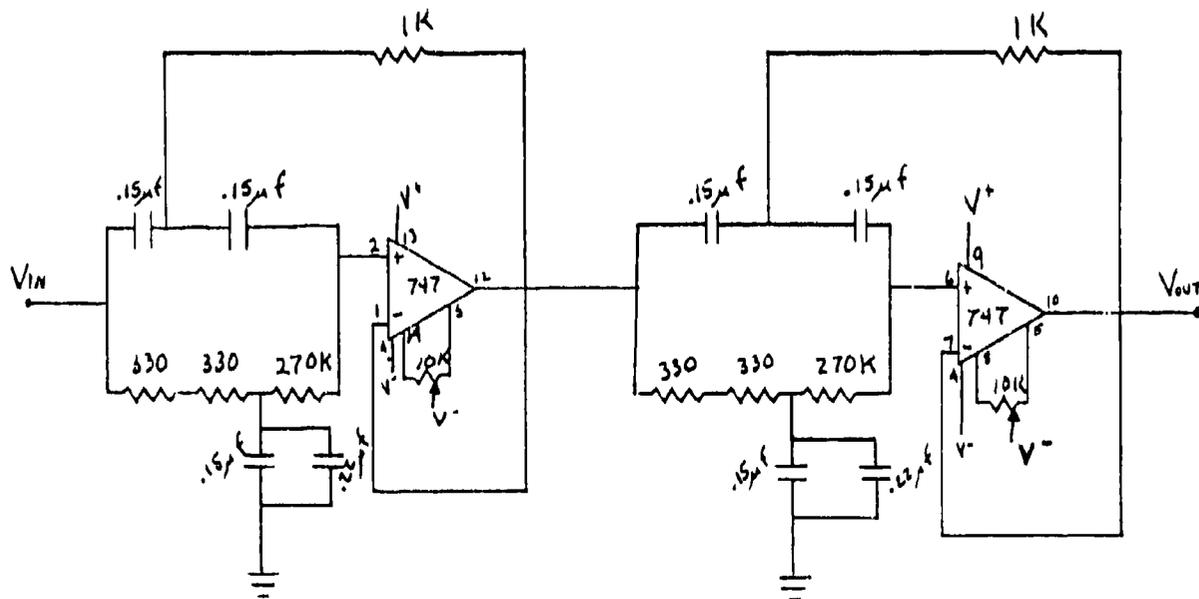
Figure 3. Band-reject filter. A voltage-controlled voltage source (VCVS) configuration is used to obtain a 60-Hz band-reject filter with a bandwidth of 60 Hz and a quality factor (Q) of 10. The output of this stage is connected to the highpass filter stage.
