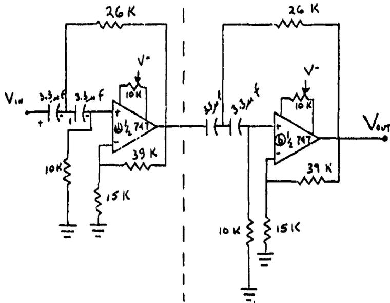
Figure 4. High-pass filter stage. A 747 Op-Amp is connected with elements to form a fourth-order high-pass filter with cutoff frequency at 3 Hz.
