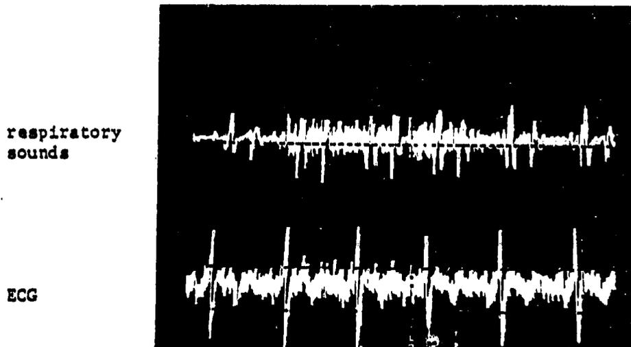
Figure 6a. Output signals recorded from the prototype system show quiet breathing from the electronic stethoscope placed at the trachea. Heart sounds may be seen through the respiration signal. The lower trace is the ECG obtained with the dry electrode system from the area of the neck.
