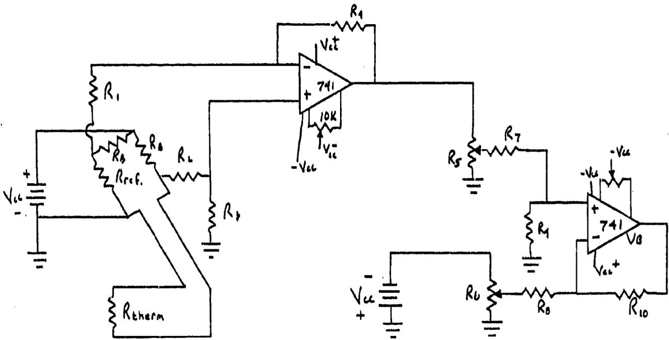
Figure 7. Surface temperature detection circuit. A bridge configuration is scaled and compared with a reference voltage. Standard 741 Op Amps are used in the design.
