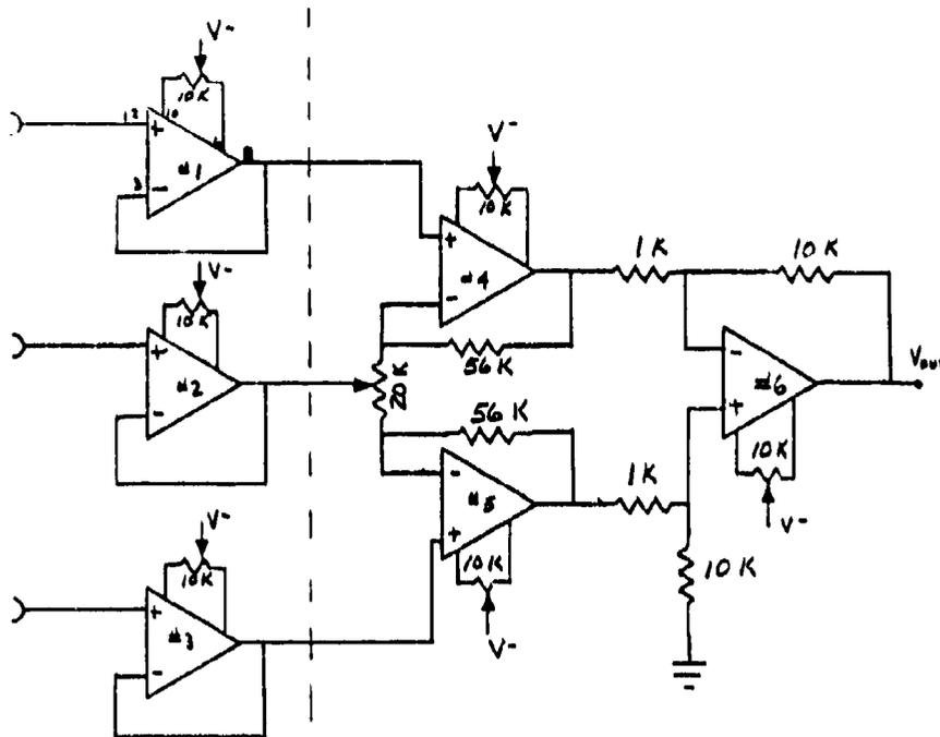
Figure 2. High impedance buffer stage is shown connected to the high common-mode rejection ratio (CMRR) stage. Amplifiers 1 - 6 are high precision FET Op Amps NSC LH0052CD. The output of the CMRR stage is input to the band-reject filter.
