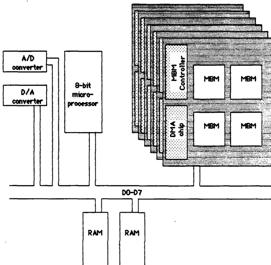
Figure 8. Modified Solid State Data Recorder
