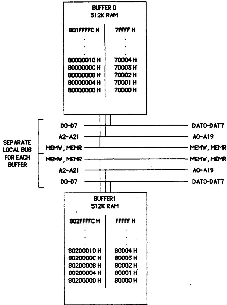
Figure 24. Ram Buffer for D0-D7 Bus
