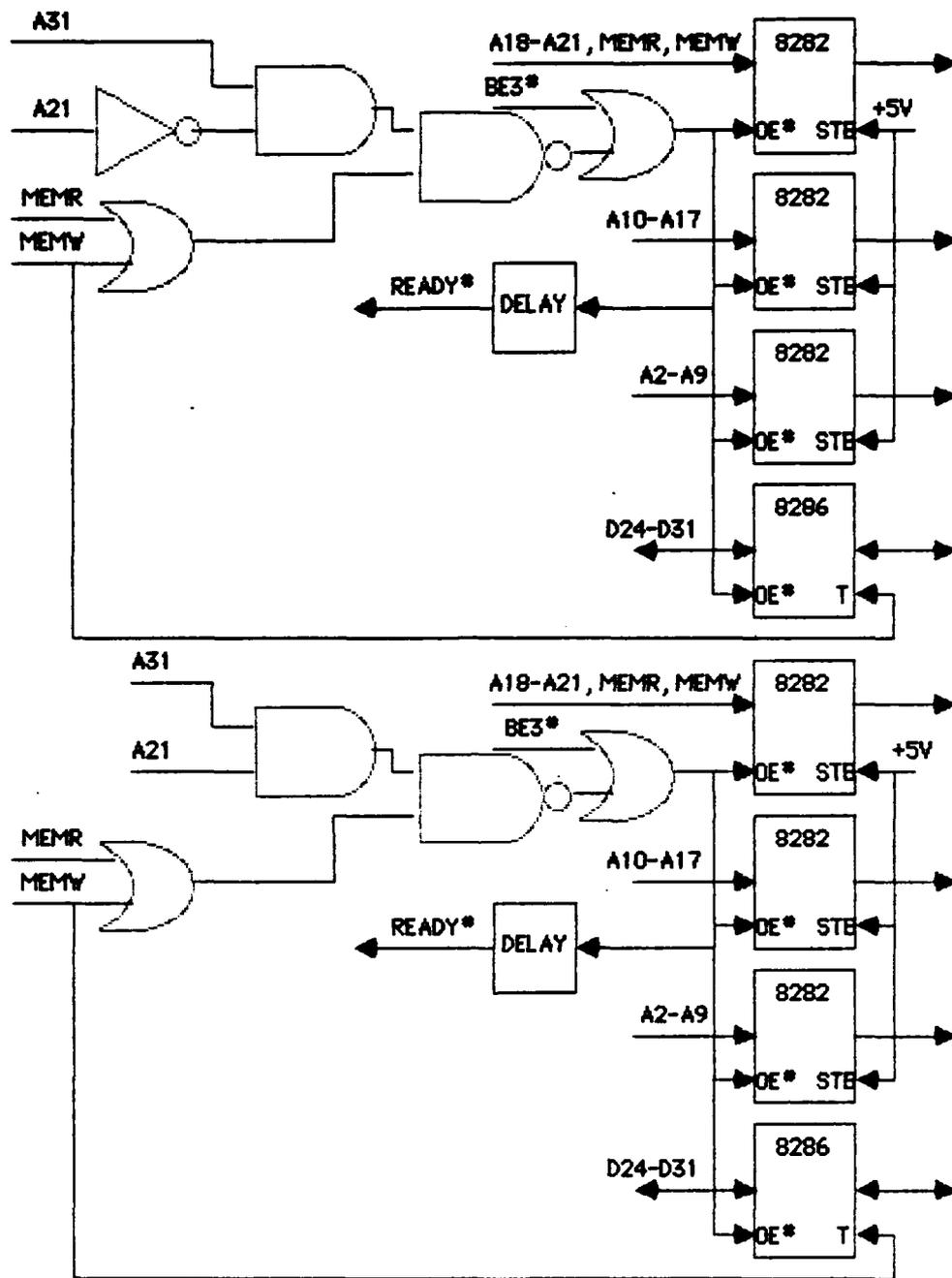
Figure 34. Microprocessor Side of MEMR/MEMW Buffer for D24-D31
