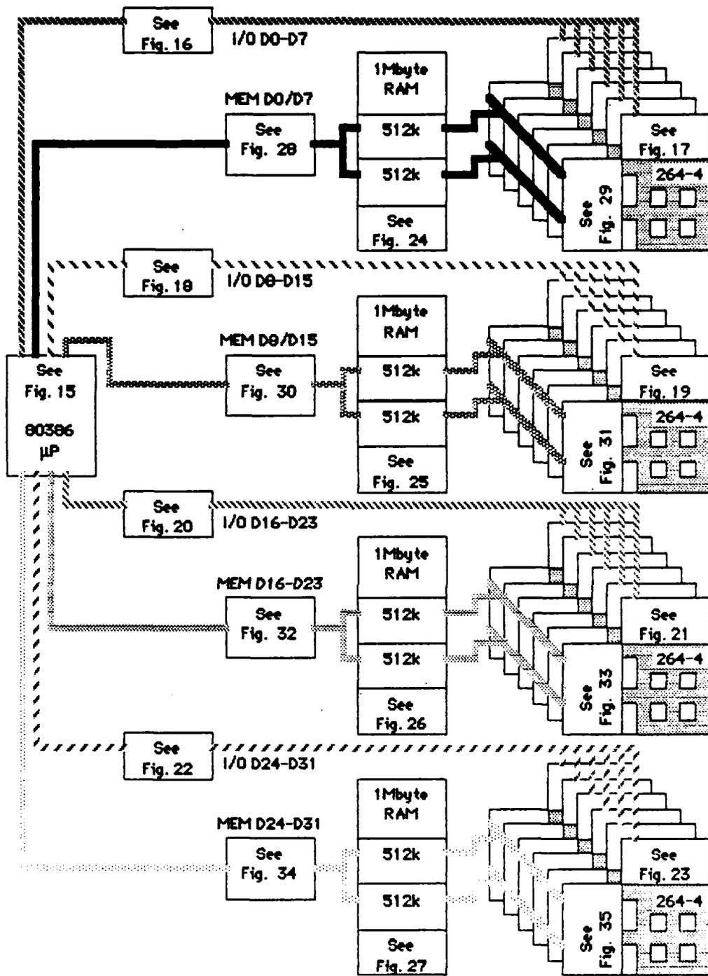
Figure 14. Advanced Solid State Data Recorder Buffer System
