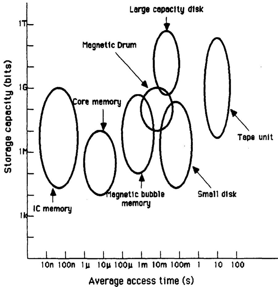
Figure 1. Storage Capacity versus Access Time
