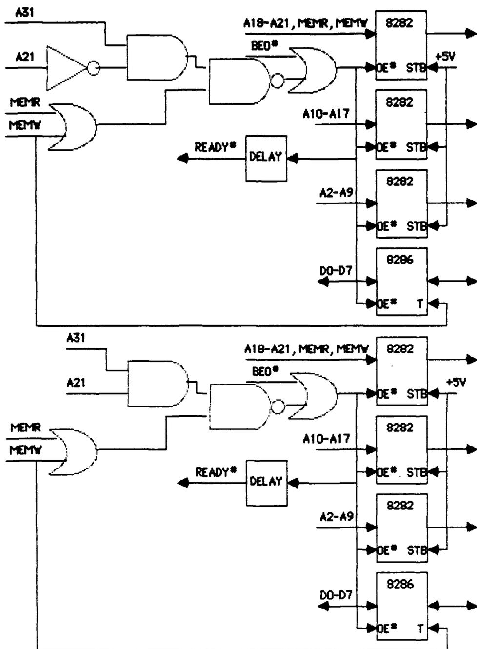
Figure 28. Microprocessor Side of MEMR/MEMW Buffer for D0-D7
