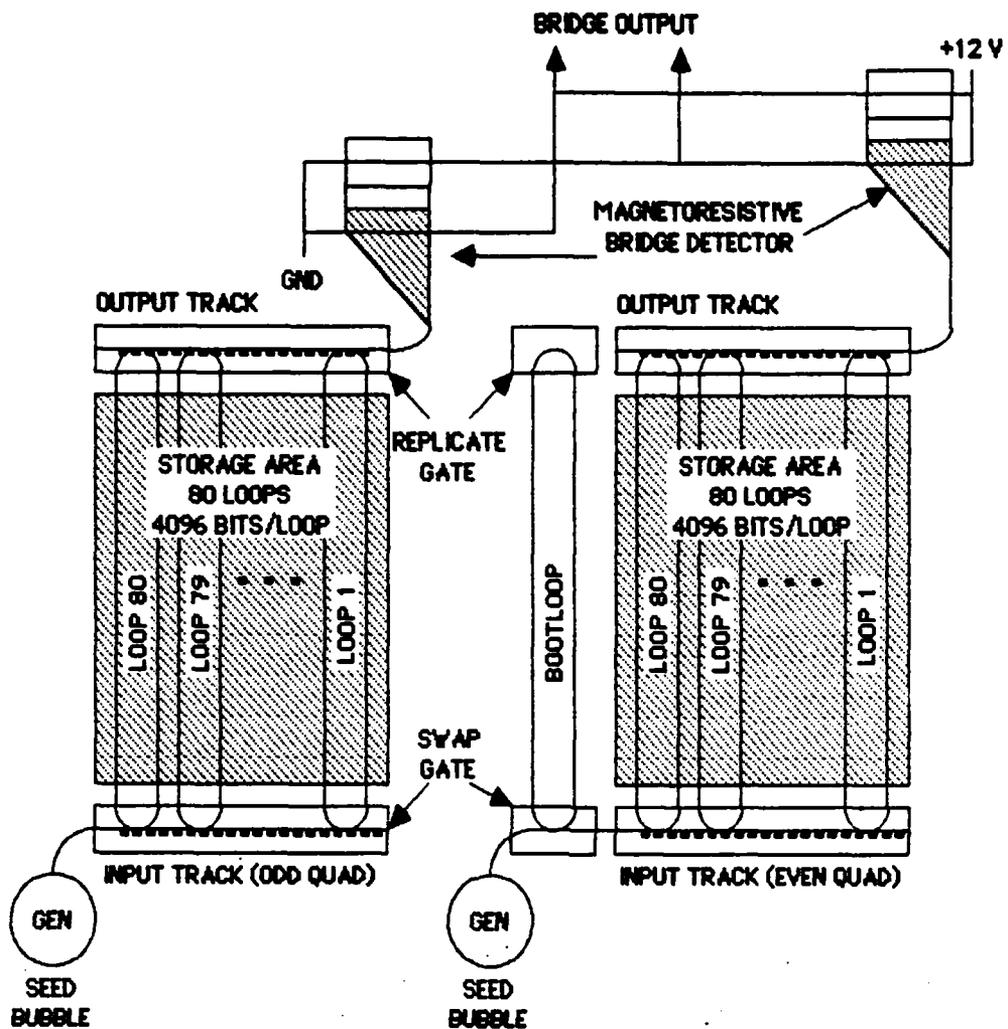
Figure 6. Magnetic Bubble Memory Architecture (One Half Shown)
