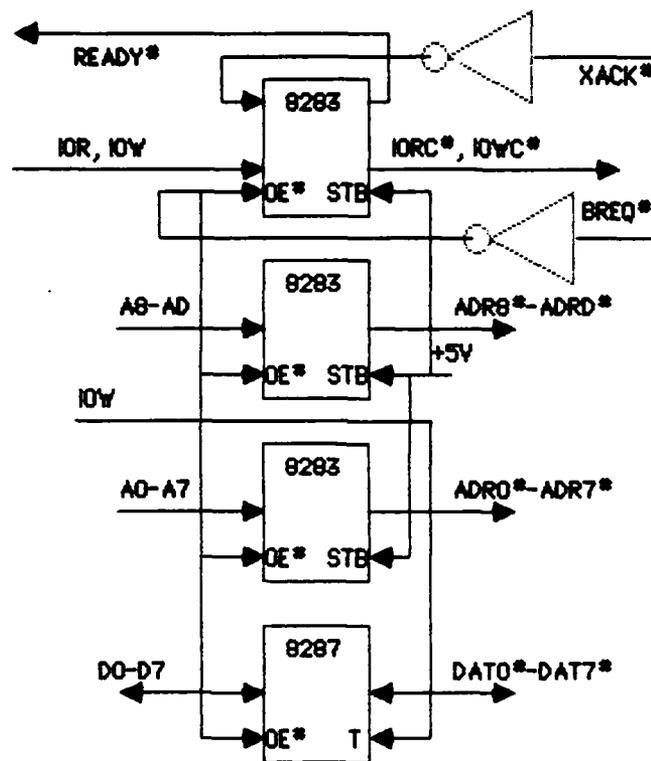
Figure 17. iSBC 264-4 Side of I/O Buffer for D0-D7 Bus
