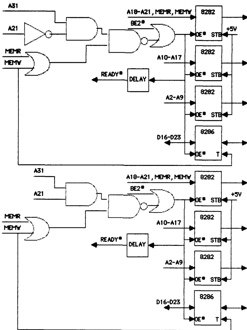
Figure 32. Microprocessor Side of MEMR/MEMW Buffer for D16-D23
