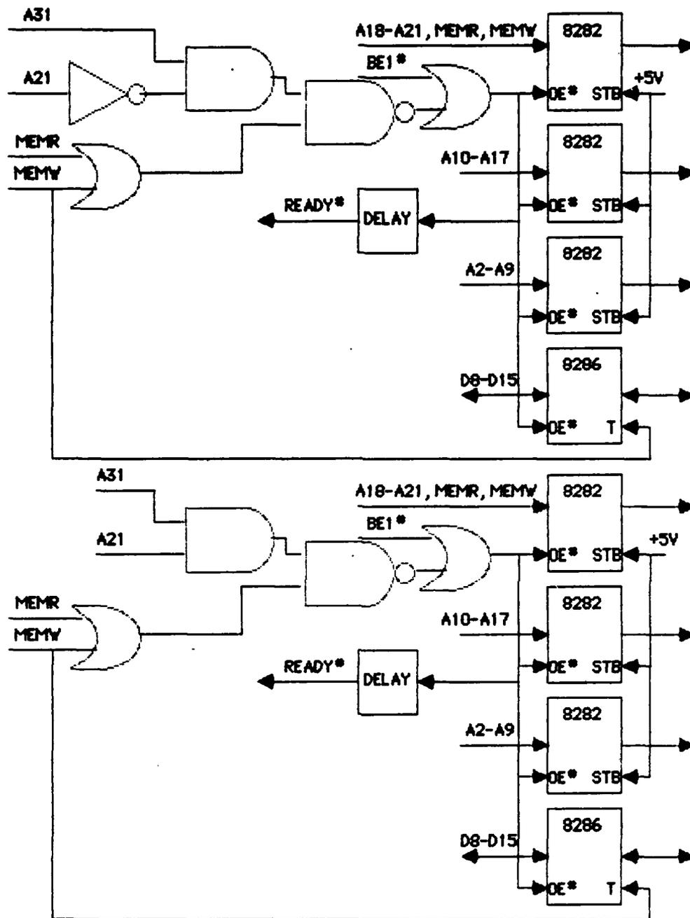
Figure 30. Microprocessor Side of MEMR/MEMW Buffer for D8-D15
