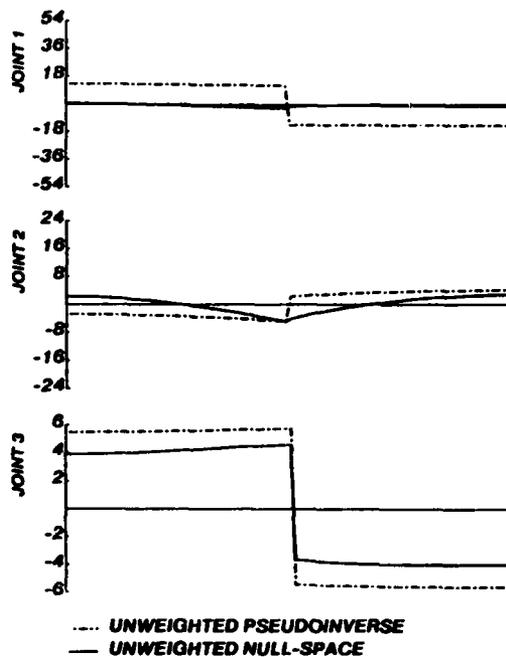
Figure 2: Torque profiles for a short movement for the pseudoinverse and null-space algorithms.
