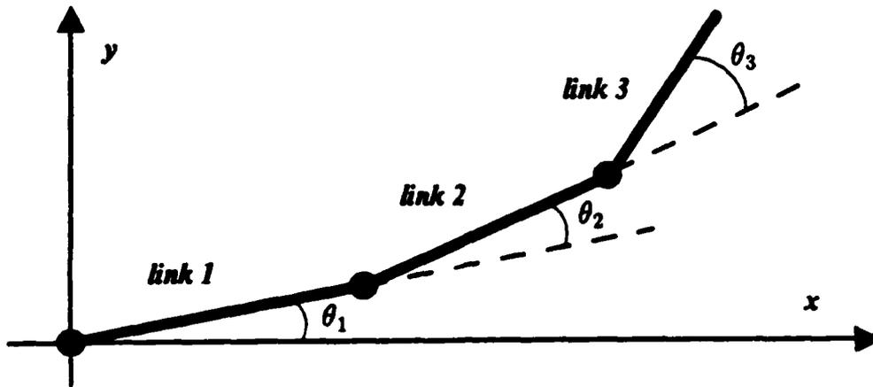
Figure 1: Geometry of the three-link planar manipulator.
