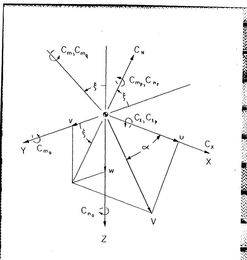
Figure 10. Aerodynamic forces and moments used in the six-degreeof-freedom simulation
