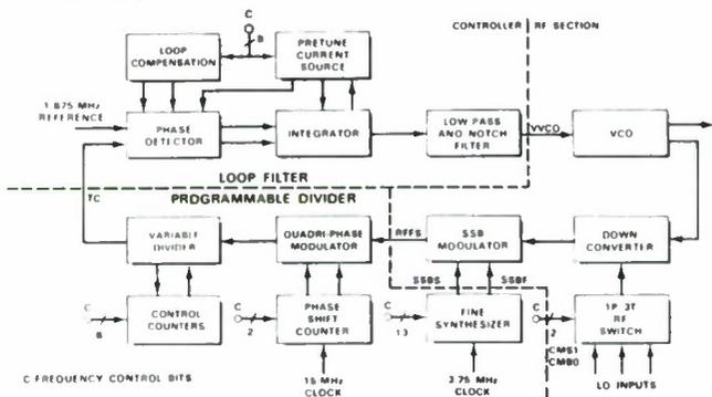
Fig. 14. Synthesizer Phase-Lock Loop Block Diagram
