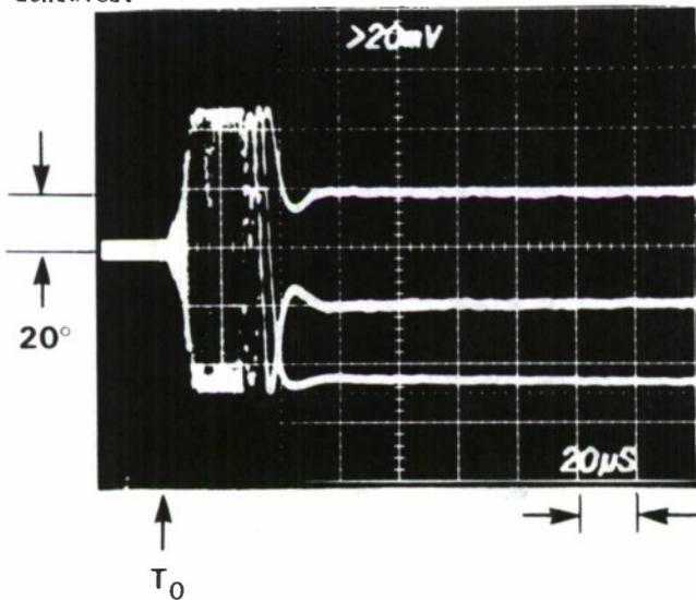
Fig. 19. Synthesizer Settling Time
