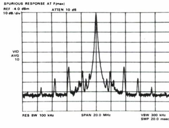
Fig. 21. FEP Frequency Synthesizer Output Spectrum
