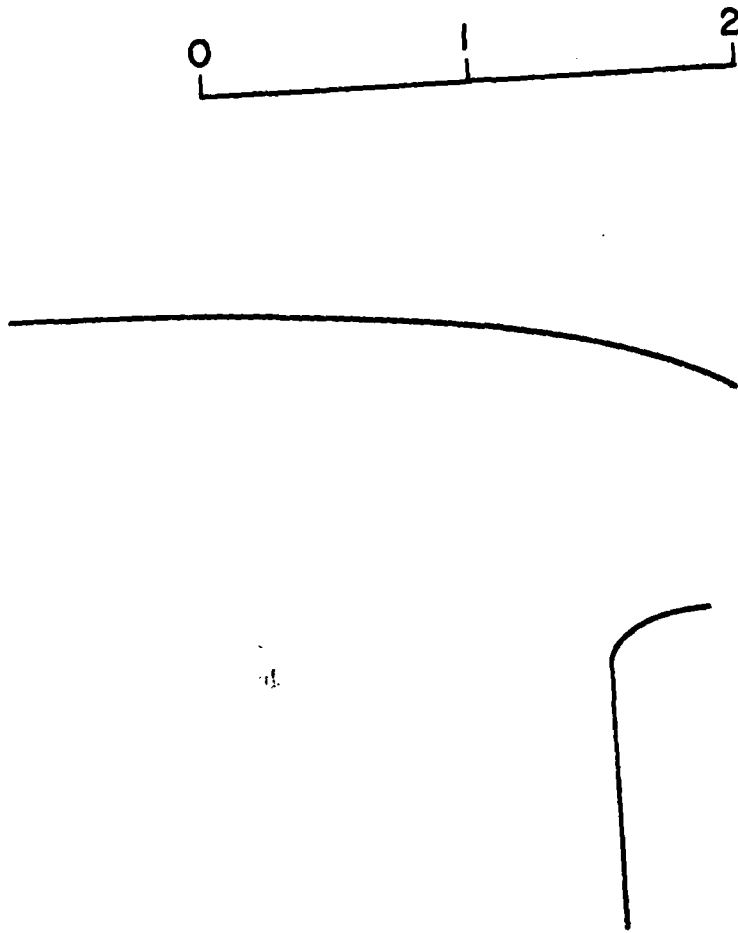
Figure 4: Computed free surface profile for the flow past a thin weir in an infinitely deep channel. The vertical scale is the same as the horizontal scale.
