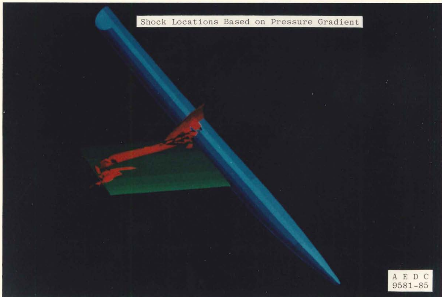
Figure 29. Wing/body shock surface, M_\infty = 0.90 , \alpha = 2 deg as determined by PLOT3D.
