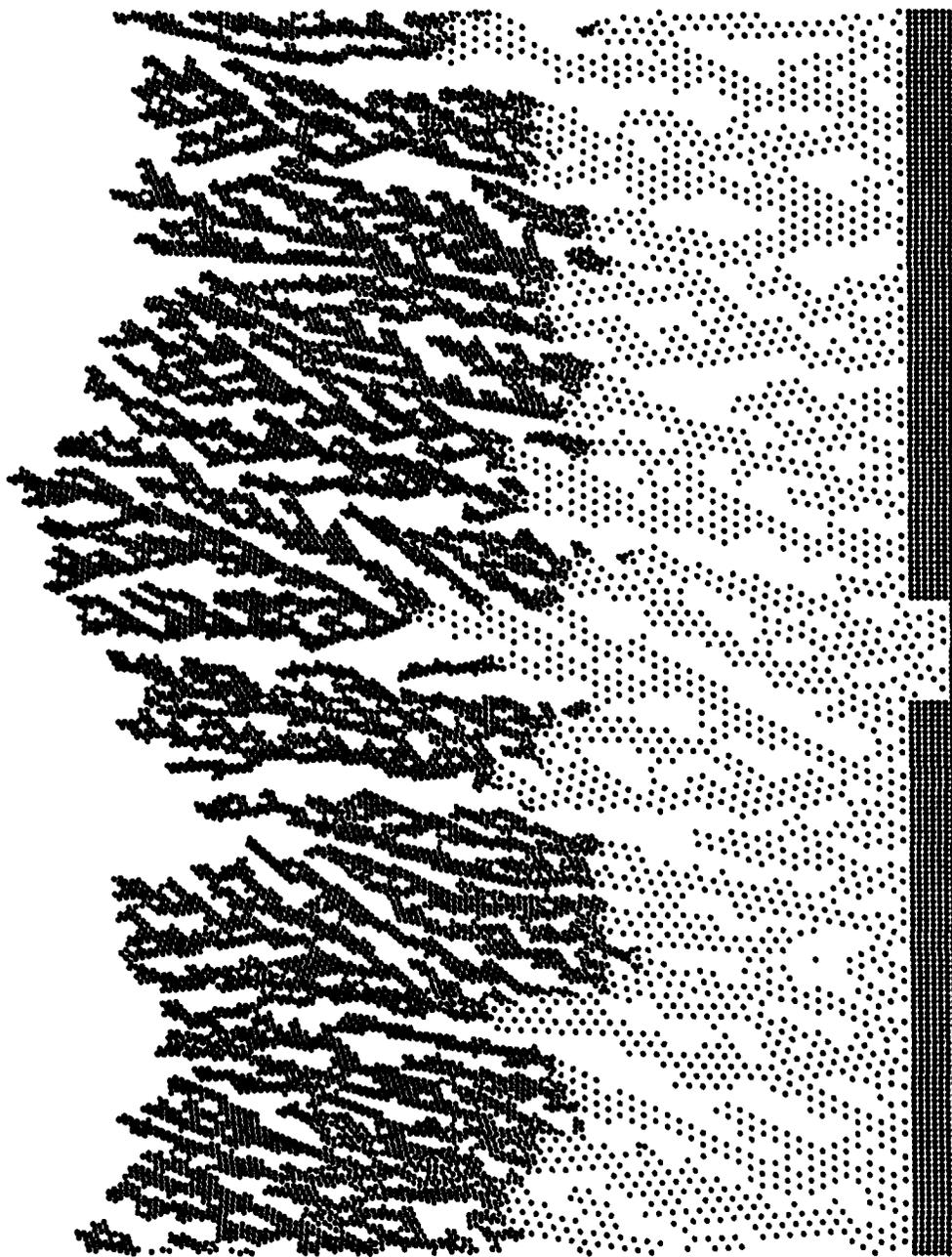
Figure 33. Multilayered Film at Normal Incidence with an Impurity in the Lower Left Hand Corner
