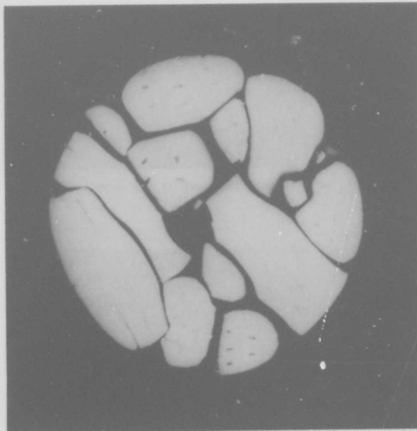
Fig. 19: Transversal cut of a M30 propellant charge after quasistatic compression at ambient temperature. The form of the originally cylindrical grains changes to fill up the available space.
