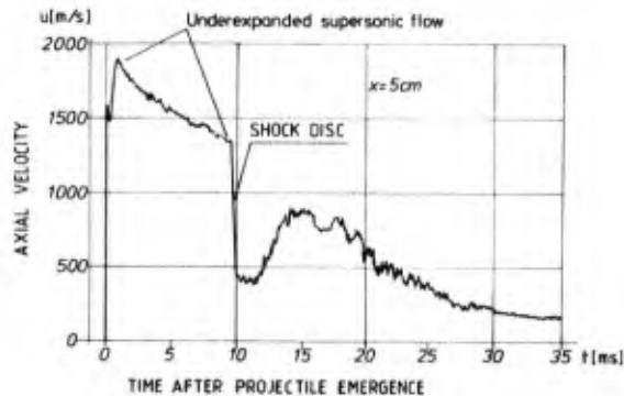
Fig. 26: Axial velocity vs. time at x = 5 cm in the muzzle blast field of a 20-mm cannon [27]
