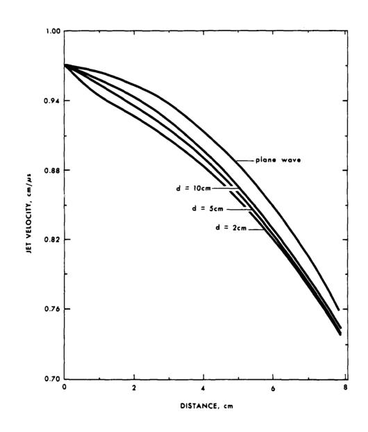
FIGURE 2 Spherically diverging wave. d is the distance, in cm, between the point of initiation and the apex of the cone.
