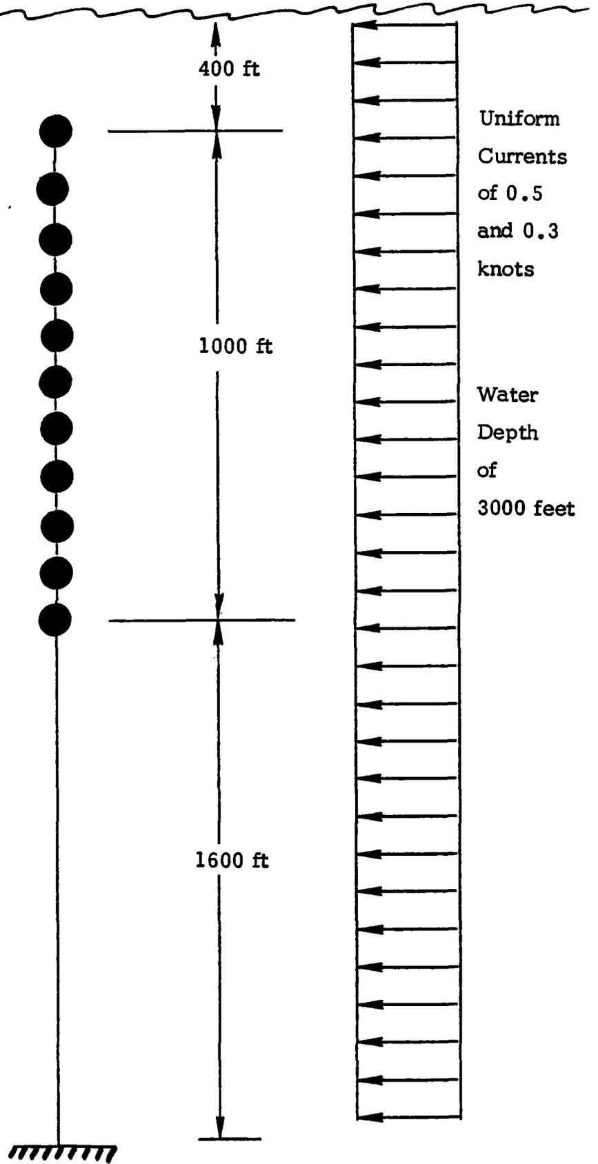
Figure 2-2. Distributed Buoy Near-Field Array Analysis Diagram
