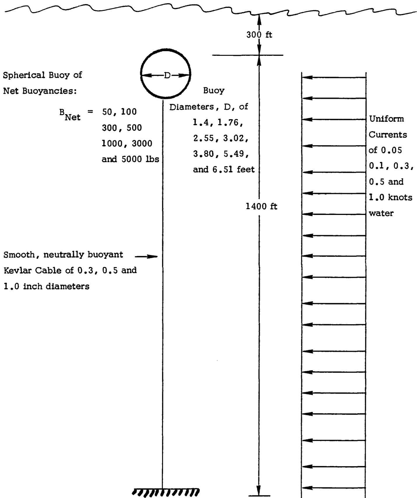
Figure 3-3. Vertical Strings Analysis Diagram
