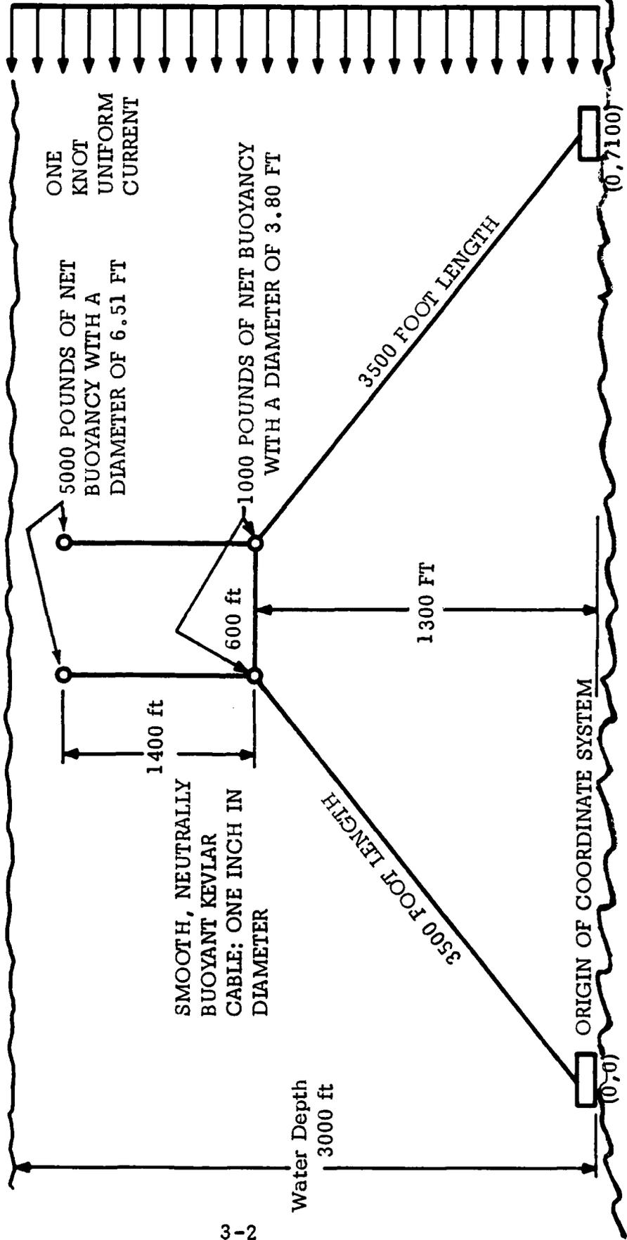
Figure 3-1. Far-Field Goal Post Array Analysis Diagram
