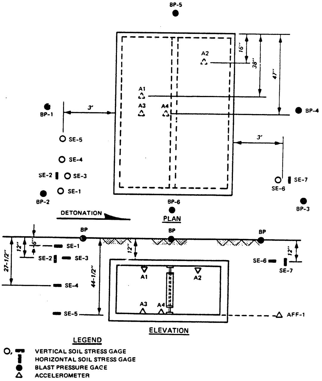
Figure 4.12. Blast pressure, soil stress, free-field acceleration, and structure acceleration gage locations for Test D.
