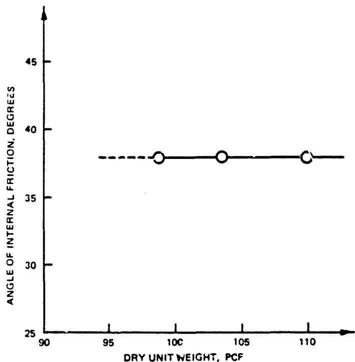
Figure 3.4. Angle of internal friction versus dry unit weight for flume sand.
