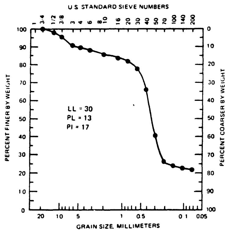
Figure 3.9. Gradation curve for clayey sand with gravel.
