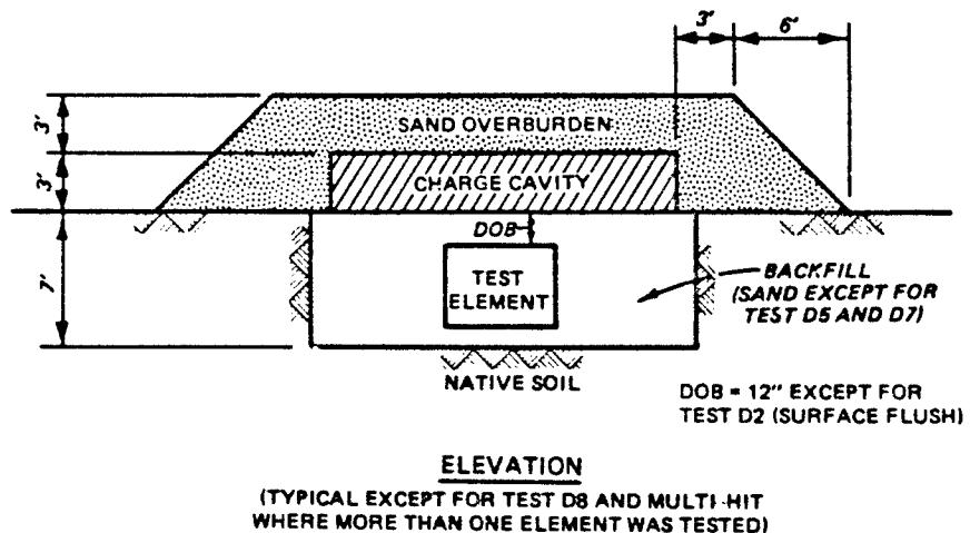
Figure 4.1. Dynamic test configuration (Sheet 1 of 2).
