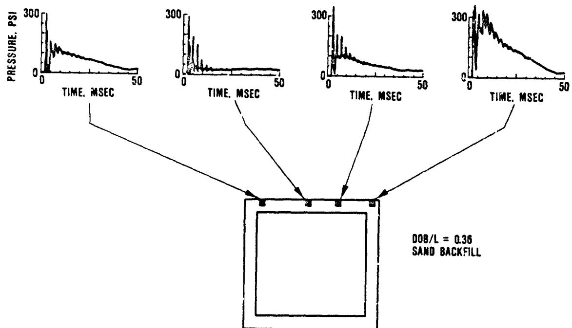
Figure 6.1. Typical dynamic test roof load distribution.
