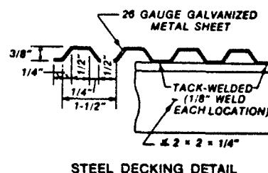
Figure 2.3. Type 1 element structural steel details.
