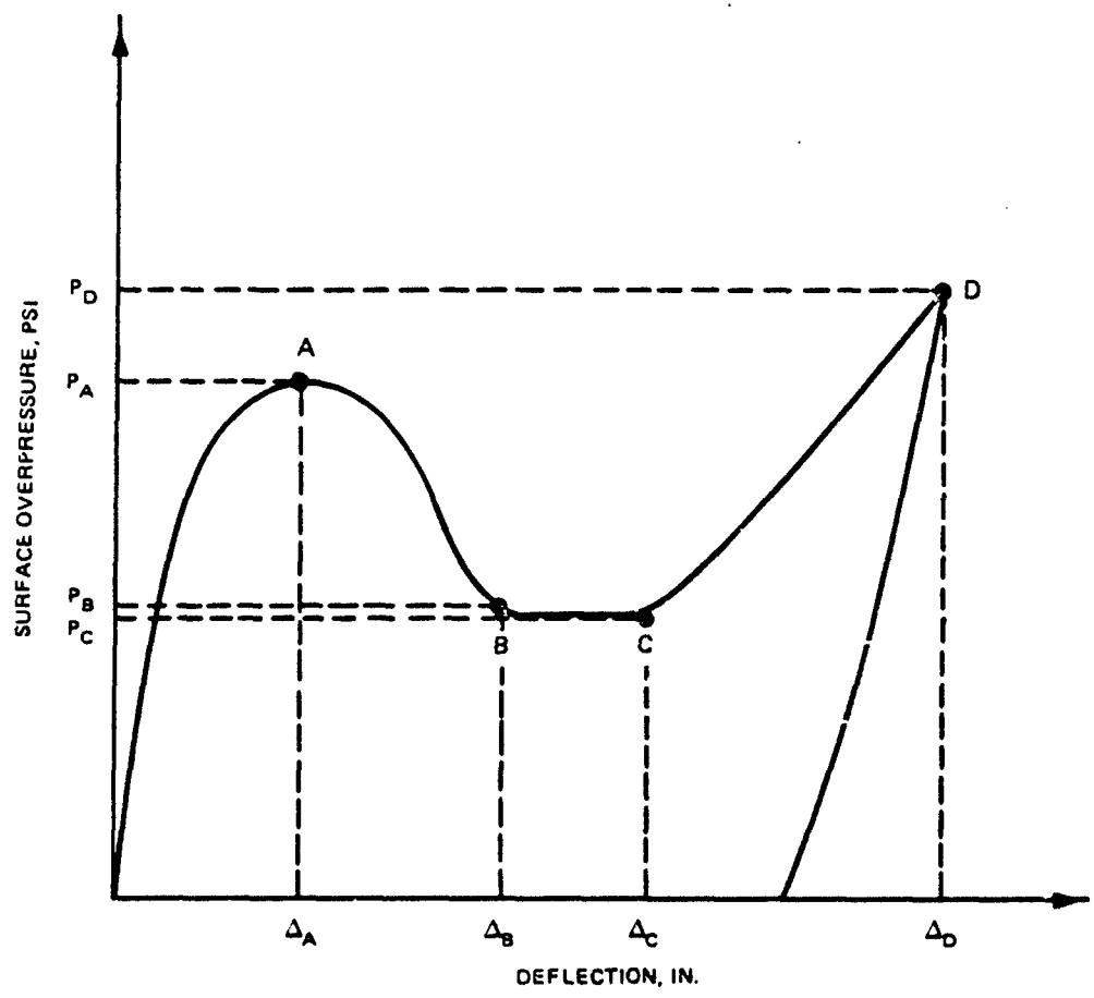
Figure 5.19. Expected load-deflection behavior for static tests.
