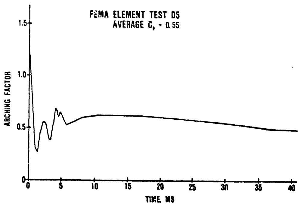
Figure 6.2. Soil arching calculated from Test D5 data.
