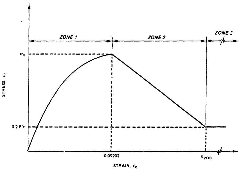
Figure 2.10. Idealized concrete stress-strain relation.
