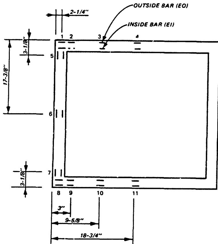
Figure 4.15. Strain gage locations for the dynamic and static Type 2 element tests.
