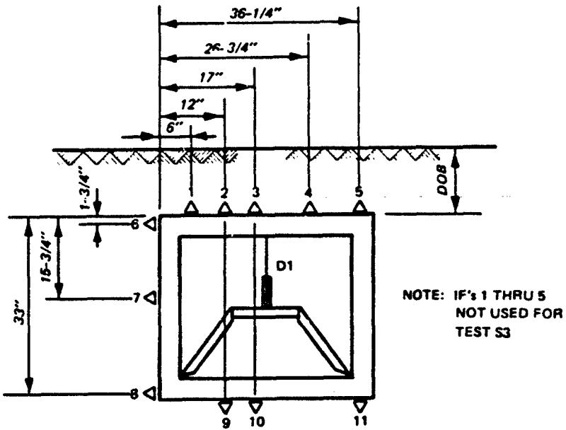
Figure 4.22. Interface pressure gage locations for Tests S4, S5, S6, and S7.
