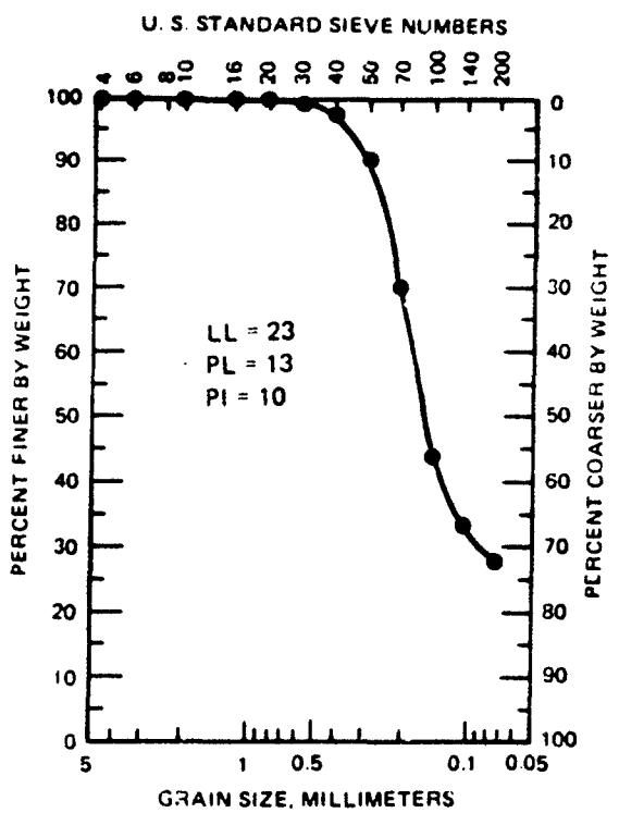
Figure 3.5. Gradation curve for red clayey sand backfill.
