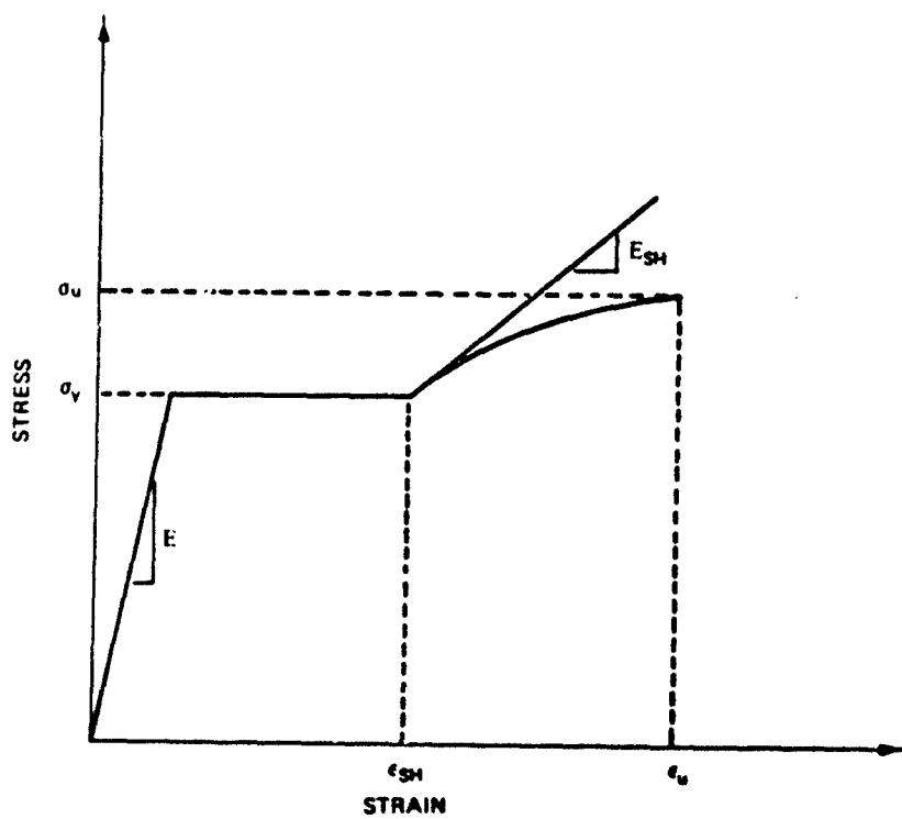
Figure 2.11. Stress-strain curve for reinforcement and structural steel.
