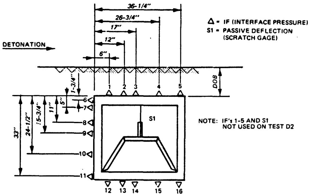
Figure 4.14. Interface pressure and deflection gage locations for Tests D2, D3, D3A, D3B, D3C, D4, D5, D6, D7, and D8.
