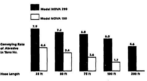
Typical conveying rates for sophisticated abrasives such as aluminum oxide, agricultural, glass beads, plastics, etc.
