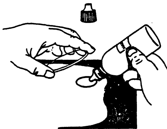
Figure 9. Adding water drops to a drawdown to test for water resistance.
