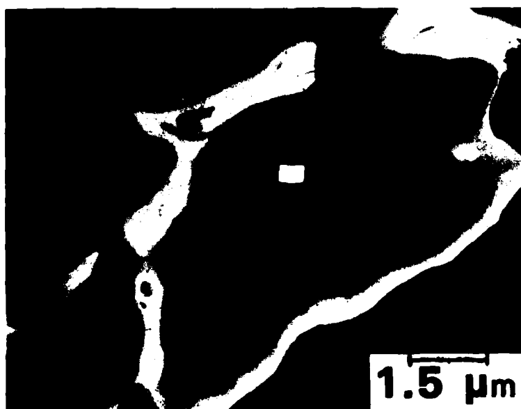
Fig. 5. STEM microstructure of a sintered CeO_2:6\% Gd_2O_3 sample showing "thick boundaries" of an amorphous silica phase. From Ref. [13].
