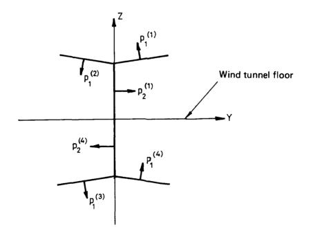
FIG. 14: IDEALISATION OF T-TAIL WITH TWO AXES OF SYMMETRY. ONLY TWO SOURCE GROUPS NEED TO BE DEFINED, THE OTHER SURFACES BEING OBTAINED BY REFLECTION. THE ARROWS INDICATE THE POSITIVE SENSES OF PRESSURE ASSUMED BY THE TOPOLOGY OF THE SOURCE GROUPS.
