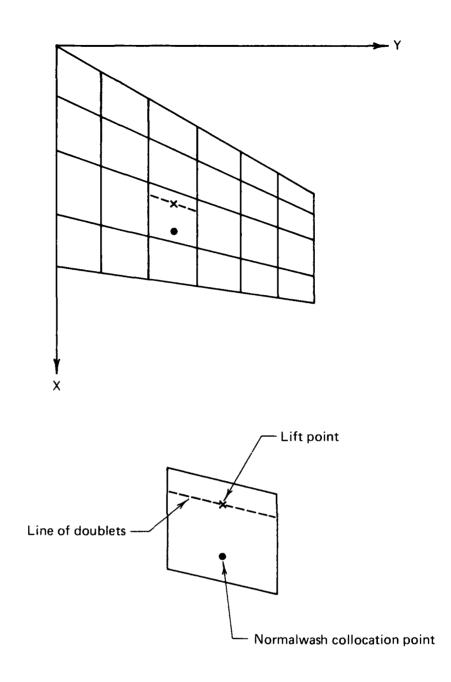
FIG. 1: EXAMPLE OF SURFACE REPRESENTATION BY PANELS AND THE FEATURES OF THE PANEL GEOMETRY.
