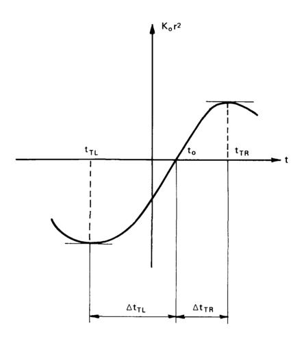
FIG. 7: DIAGRAM ILLUSTRATING THE DEFINITIONS OF  $\triangle t_{TL}$ ,  $\triangle t_{TR}$ ,  $t_{TL}$ ,  $t_{TR}$  AND  $t_{o}$  IN RELATION TO THE CURVE OF  $K_{o}r^{2}$  FOR PANELS THAT ARE PERPENDICULAR TO EACH OTHER.
