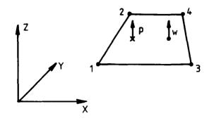
FIG. 11: DIAGRAM SHOWING POSITIVE SENSE OF PRESSURE p AND NORMALWASH w IN RELATION TO THE TOPOLOGY OF THE PANEL.
