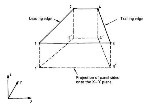
FIG. 8: DIAGRAM SHOWING NODE NUMBERING SCHEME AND OTHER FEATURES PERTAINING TO THE DEFINITION OF A GROUP. THE NUMBERS 1, 2, 3 AND 4 REFER TO THE NODES.
