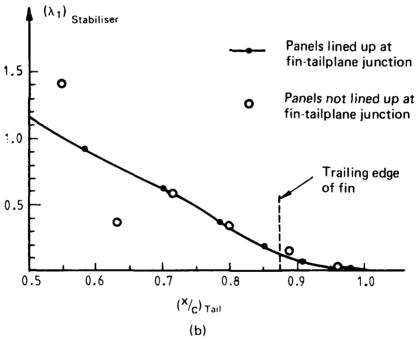
FIG. 18: PLOT OF THE NONDIMENSIONAL PRESSURE DISTRIBUTION  $\lambda_1$  NEAR THE FIN-STABILISER JUNCTION FOR STARK'S T-TAIL FOR THE FIN YAW MODE (MODE F<sub>1</sub>). PRESSURES ARE SHOWN FOR BOTH THE FIN AND STABILISER AND WERE OBTAINED FOR K = 0 & M = 0.
