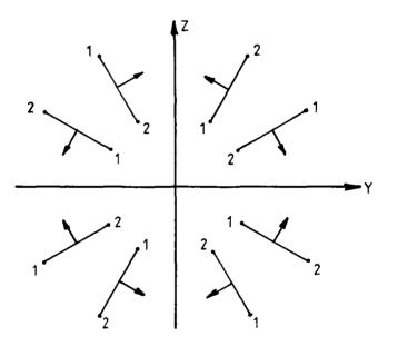
FIG. 12: DIAGRAM SHOWING POSSIBLE PANEL TOPOLOGIES IN EACH QUADRANT AND THE ASSOCIATED DIRECTION OF POSITIVE PRESSURE.
