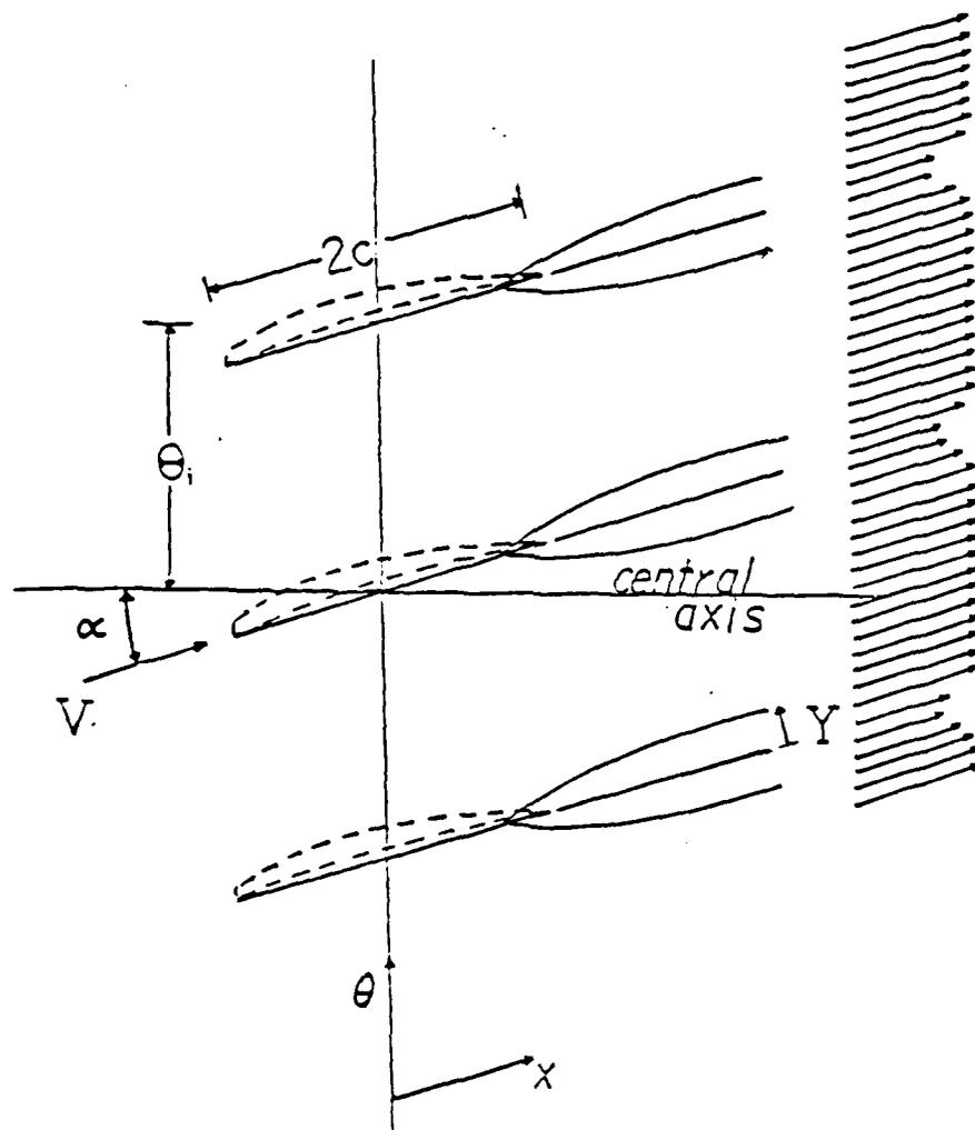
Figure 1. Schematic of Flow About an Infinite Cascade
