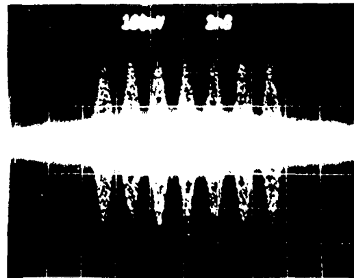
Fig. 4. Analyzer output in response to 7 CW tones from 3.4 to 4.0 GHz.
