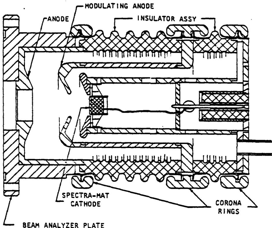
Figure 2. Electron gun design. a) cathode, b) modulating anode, c) anode.
