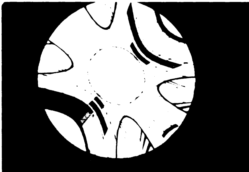
Plate 8. Test pattern (Plate 3) resampled the same as sample B in Plate 7. Geometrical effect of transformation is apparent, including apparent defocusing away from central region
