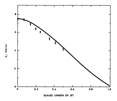
FIGURE 8 Velocity gradient within the MRL jet as a function of scaled length of jet. The solid line is the prediction of the model, the experimental points are from recent work by M.C. Chick [15].
