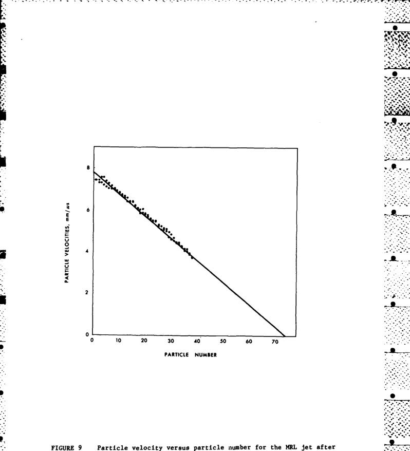
IGURE 9 Particle velocity versus particle number for the MRL jet after breakup. The different data points represent two experiments from recent work by M.C. Chick [15].
