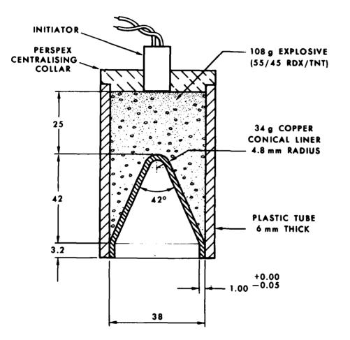
FIGURE 6 The MRL 38 mm shaped charge. All lengths in mm.
