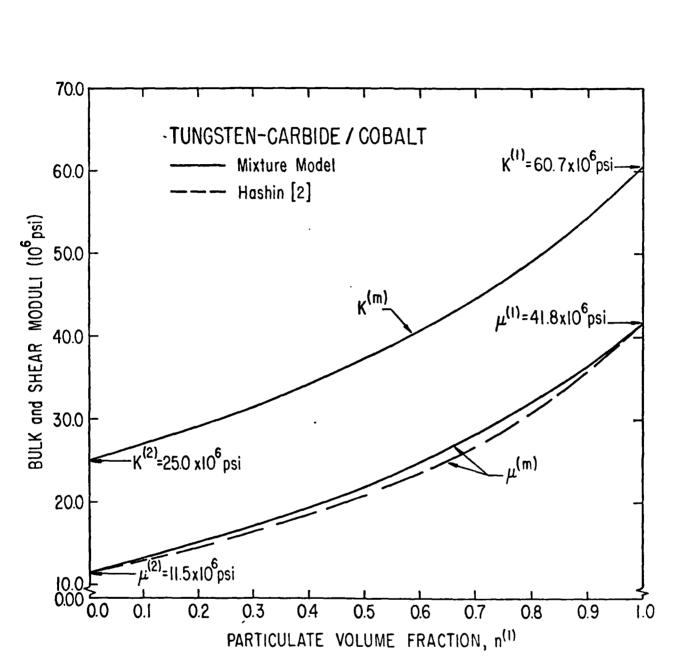
Figure 3. Bulk and Shear Moduli as a Function of Particulate Volume Fraction.
