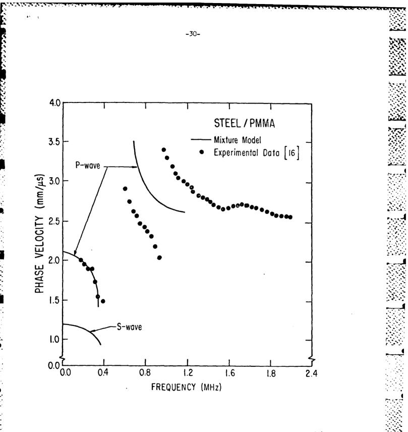
Figure 5. Phase Velocity as a Function of Frequency in Steel/PMMA Composite.
