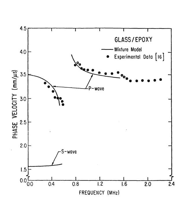
Figure 4. Phase Velocity as a Function of Frequency in Glass/Epoxy Composite.
