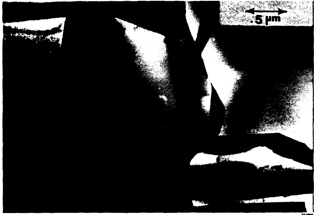
FIGURE 11-B. TEM MICROGRAPHS OF STACKING FAULTS IN 6-MICRON GaAs FILM GROWN ON \langle 01\bar{1}2 \rangle \text{Al}_2\text{O}_3 .
