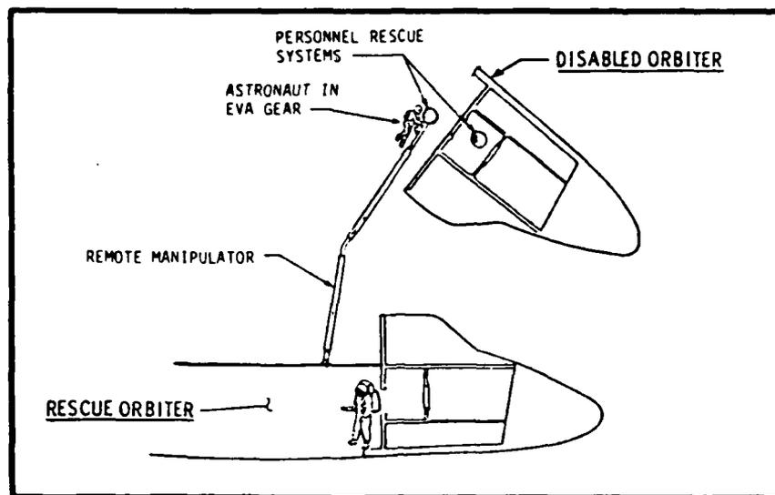
Figure 1.2. PRE Transfer via Remote Manipulator Arm (1:202)
