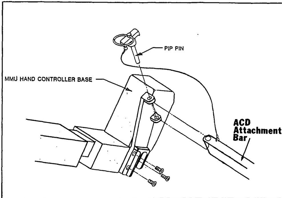
Figure 3.3. Detail of MMU/ACD Attachment
