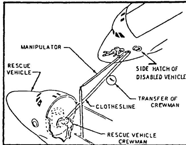
Figure 1.3. PRE Transfer via Clothesline Trolley (1:203)
