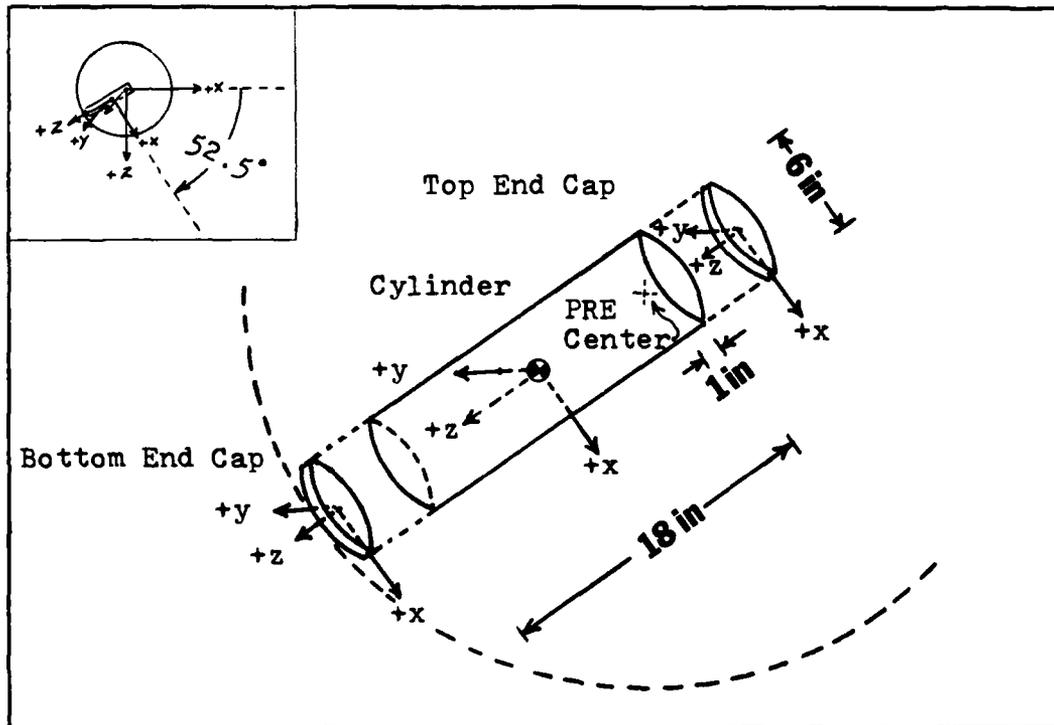
Figure 4.5. Portable Oxygen System Components and Principal Axes
