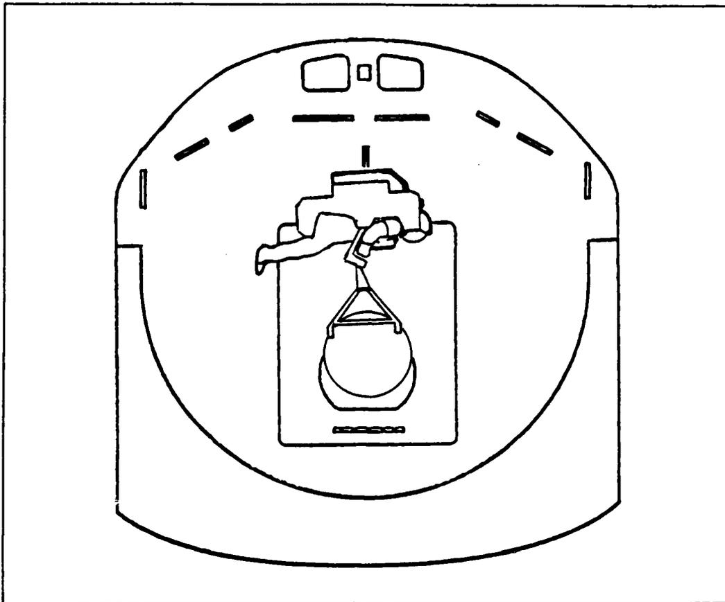
Figure 6.1. IRV Attached to Forward Bulkhead of Stranded Orbiter
