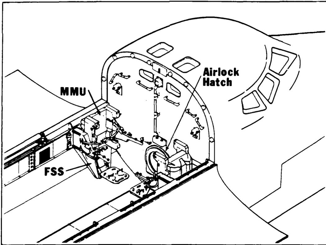
Figure 2.5. Manned Maneuvering Units (MMU) Mounted in Flight Support Stations (FSS) (26:2)
