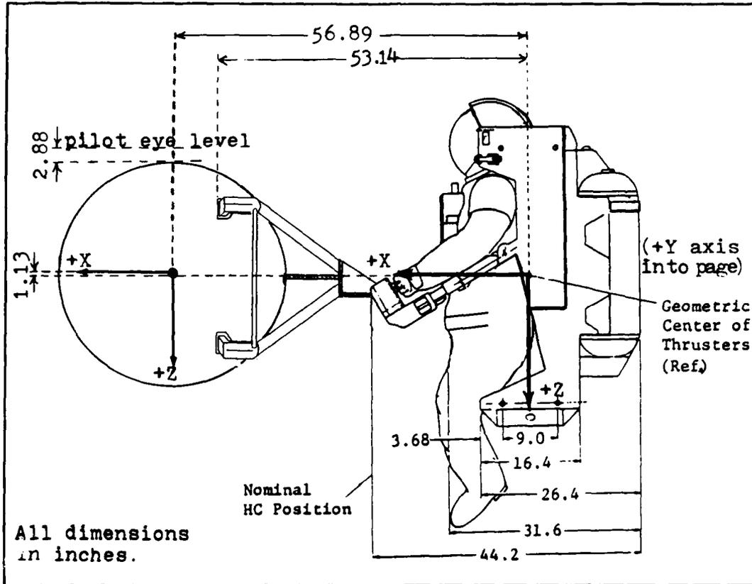
Figure 4.1 IRV Dimensions and Coordinate Systems (18:2.4-154)
