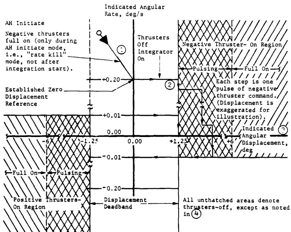
Figure 2.7. Automatic Attitude Hold System Control Logic (9:2-35)
