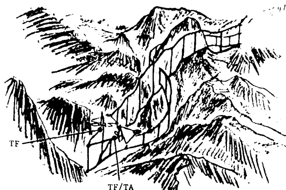
Figure 1. Terrain Following (TF) and Terrain Following/Terrain Avoidance (TF/TA) Trajectories
