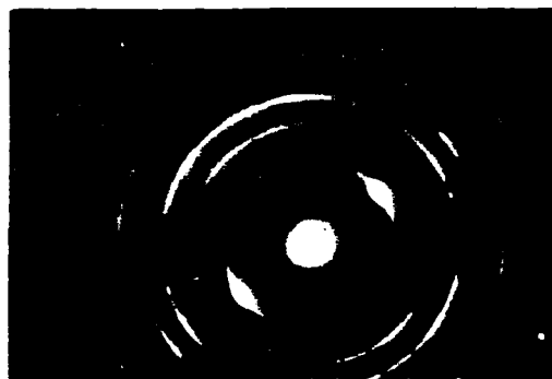
High voltage transmission electron micrographs of chromium electrodeposited at 55°C. Sample was tilted around an axis along the microcrack. Missing 200 reflection and discontinuous arcs are characteristic of a 110 fiber texture parallel to the film thickness direction.
