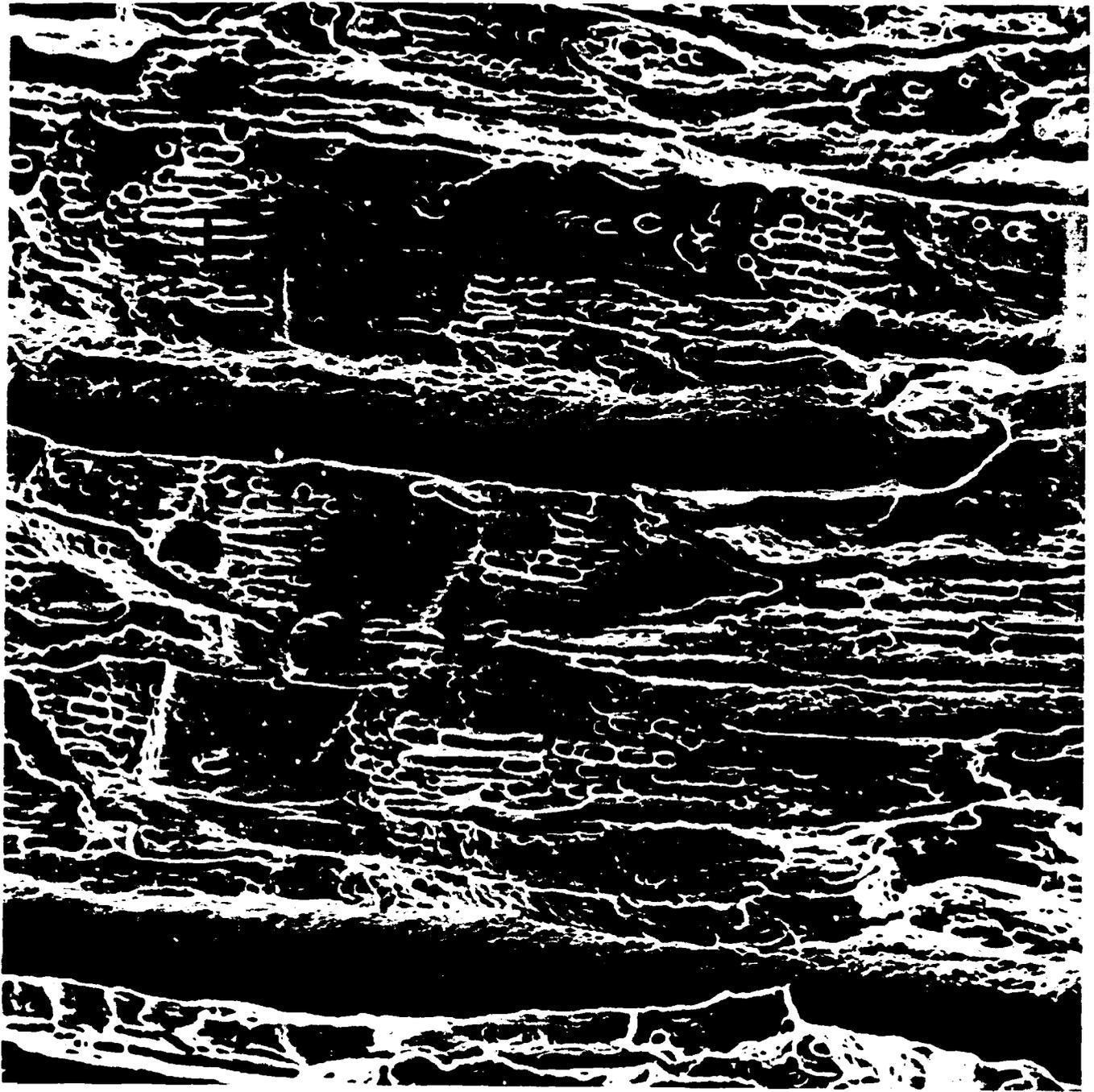
Figure 9. Fracture surface in mercury under fixed load conditions for 1100-1,  $K > \sim 8 \text{ MPa}\sqrt{\text{m}}$ . The marker is  $100 \mu\text{m}$ .
