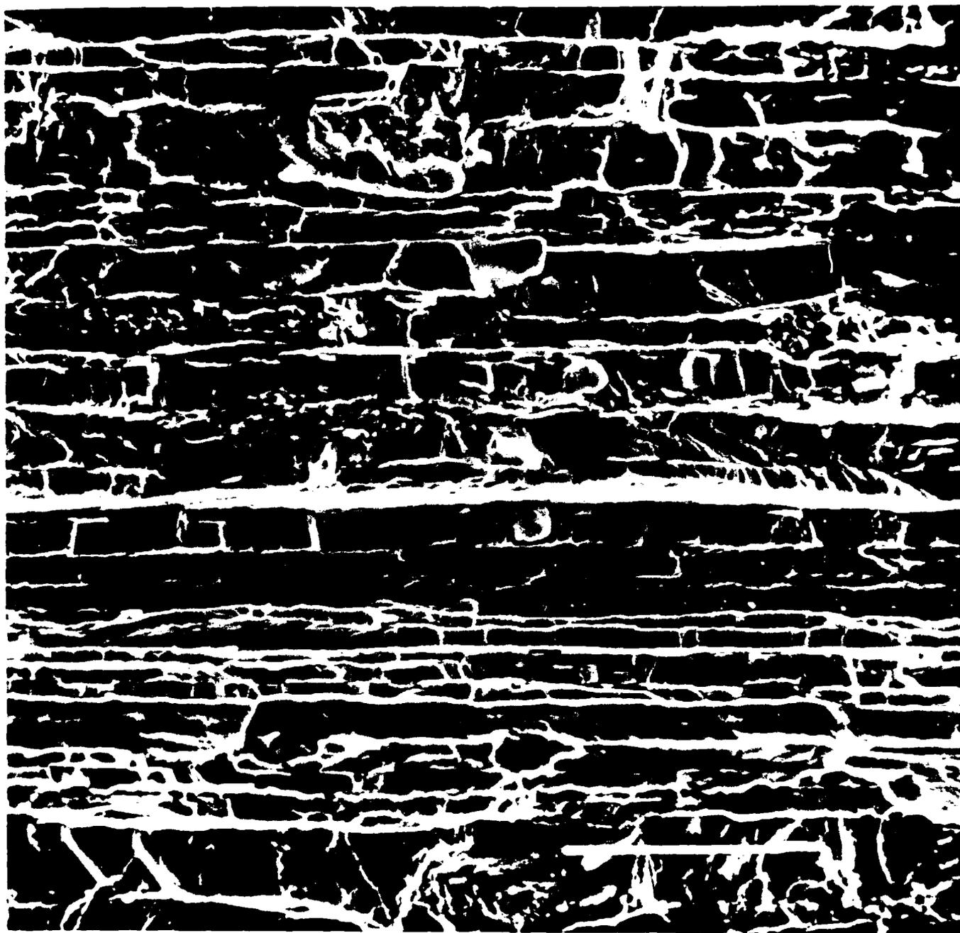
Figure 14. Fracture appearance in mercury under cyclic loading conditions for 7075-T651,  $\Delta K > \sim 3 \text{ MPa}\sqrt{\text{m}}$ , 5 Hz or 30 Hz. The marker is 50  $\mu\text{m}$ .
