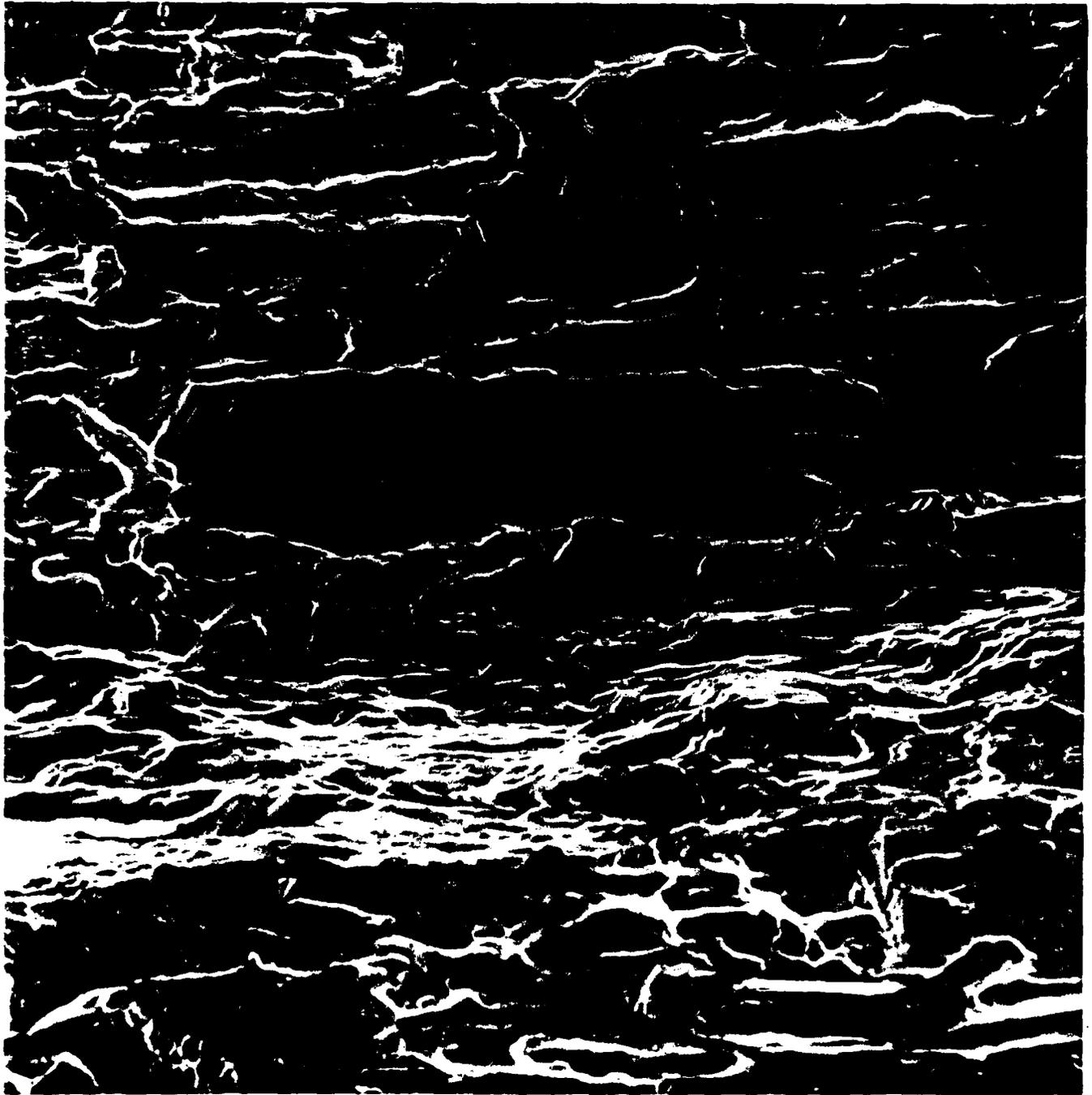
Figure 11. Fracture appearance in mercury under fixed displacement conditions for 1100-0,  $K > \sim 8 \text{ MPa}\sqrt{\text{m}}$ . The marker is 100  $\mu\text{m}$ .
