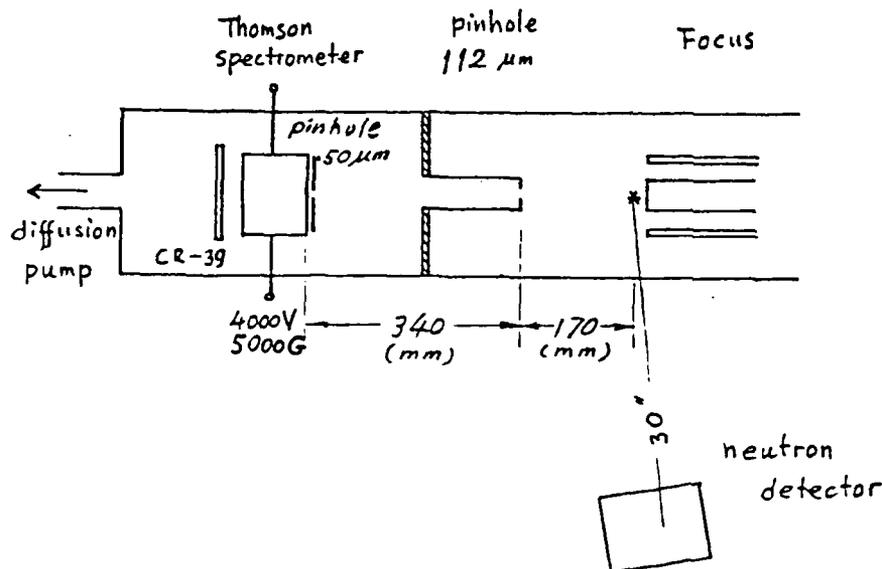
The experimental arrangement for tests with the high resolution magnetic analyzer ( 7-12.5 kG, edge focusing,  $dE/E$  0.5%, 10 ms opening valve ) is described in the literature:
