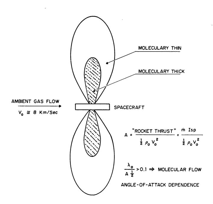
FIGURE 2-2: MOLECULAR FLOW OF AMBIENT GAS
