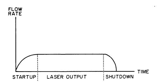
FIGURE 2-5: STARTUP AND SHUTDOWN TRANSIENTS
