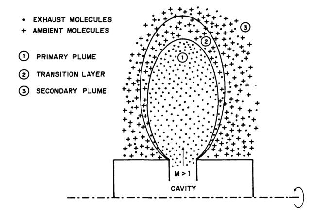
FIGURE 3-1: SCHEMATIC DESCRIPTION OF LASER EXHAUST FLOW FIELD
